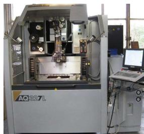
Fig. 3. Workstation with wire electrical discharge machine Sodick AQ327L
