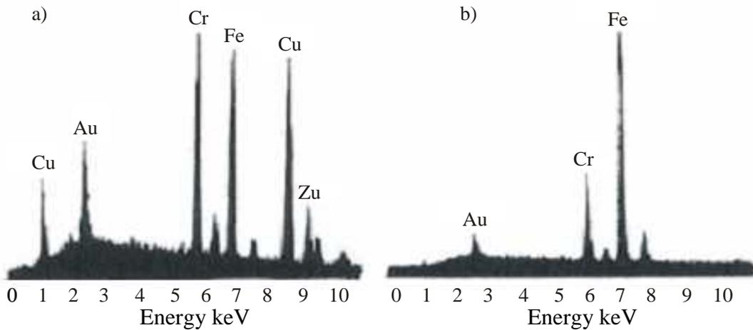
Fig. 6. a) Analysis of X-ray chemical composition in crater b) Analysis of the composition of surface around the craters
