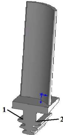
Fig. 1. A multi-trapezoidal-type blade root.1) is typically found cracks, 2) recorded only traces of corrosion
