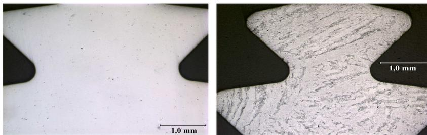
Fig. 4. Outer surfaces of the test item. The material of nonmetallic inclusions visible principally in the form of sulphides and oxides of spaced spot. Unetched state. Light microscopy
