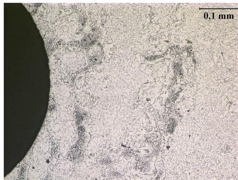
Fig. 5. Cross-section. Heterogeneous ferritic structure with a strong segregation (band) chromium carbides
