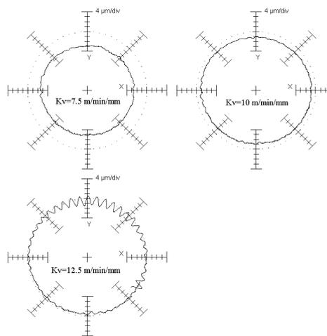
Fig. 2. Circular and radial deviation of the measured circular tests with different position loop gains  $K_v$  ( $R=10$  [mm],  $v=5$  [m/min],  $a=10$  [ $m/s^2$ ],  $T=0.001$  [s], CCW, velocity feed-forward active) (.....) nominal contour, (-----) actual contour
