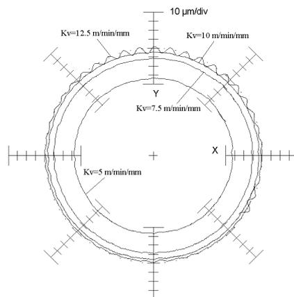
Fig. 3. A summary polar diagram of circular and radial deviation of the measured circular tests with different position loop gains  $K_v$  ( $R=10$  [mm],  $v=5$  [m/min],  $a=10$  [ $m/s^2$ ],  $T=0.001$  [s], CCW, velocity feed-forward active), (.....) nominal contour, (-----) actual contour
