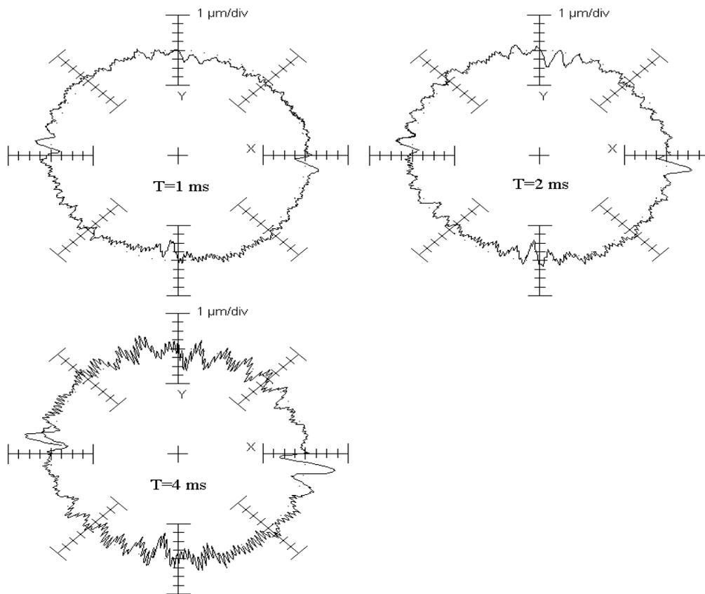
Fig. 4. Circular deviation of the measured circular tests with different sampling periods ( $R=10$  [mm],  $v=5$  [m/min],  $a=10$  [m/s<sup>2</sup>],  $K_v=10$  [(m/min)/mm] ]=166.7 [1/s], CW, velocity feed-forward active) (.....) nominal contour, (-----) actual contour
