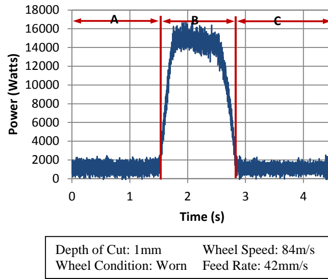
Fig. 2. Example of power trace of digital drive signal
