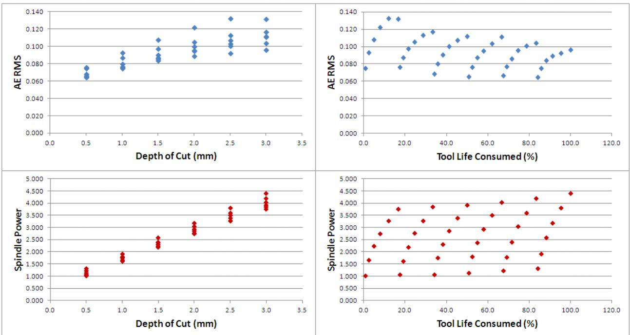
Fig. 9. All test results for spindle power and AE RMS. Note; tool life consumed is a measure of metal removed by tool
