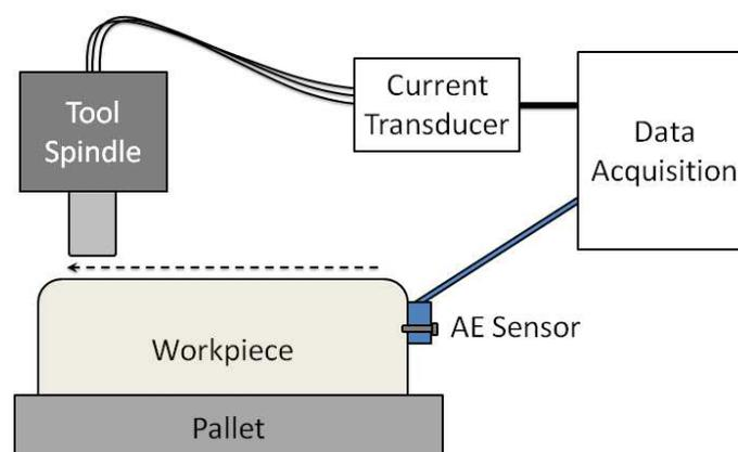
Fig. 6. Experimental set up for profile milling trials
