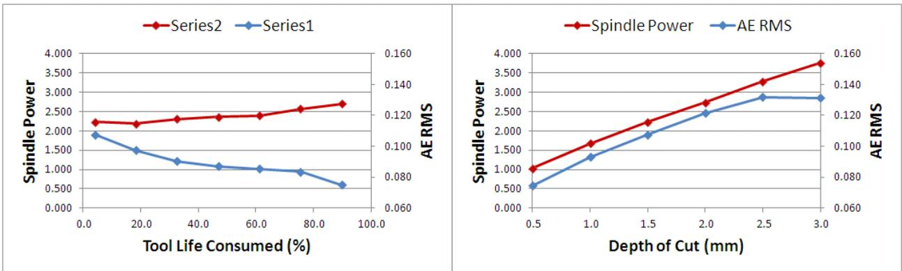
Fig. 8. Observed relationships between depth of cut and tool life from experimental data. Note; tool life consumed is a measure of metal removed by tool
