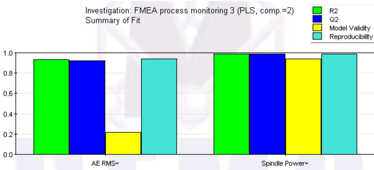
Fig. 11. Summary of fit of data in PLS model. Note that R2 is the coefficient of multiple determination, where a value near to 1 indicates a good fit of the data in the model. Q2 is the fraction of the variation of the response predicted by the model, where a value near 1 indicates good predictability of the model
