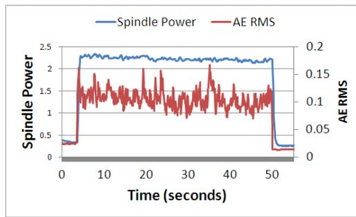
Fig. 7. Sensor signal time graph for 1.5mm radial depth of cut and a new tool. Entry to cut can be seen at approximately 4 seconds on the x axis, and exit from cut can be seen at approximately 50 seconds
