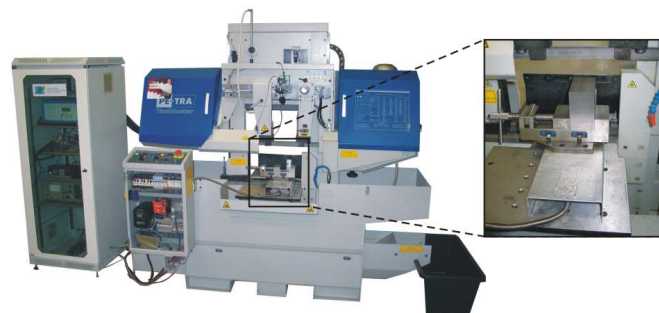
Fig. 1. Multisensory dual column band saw machine used in the research
