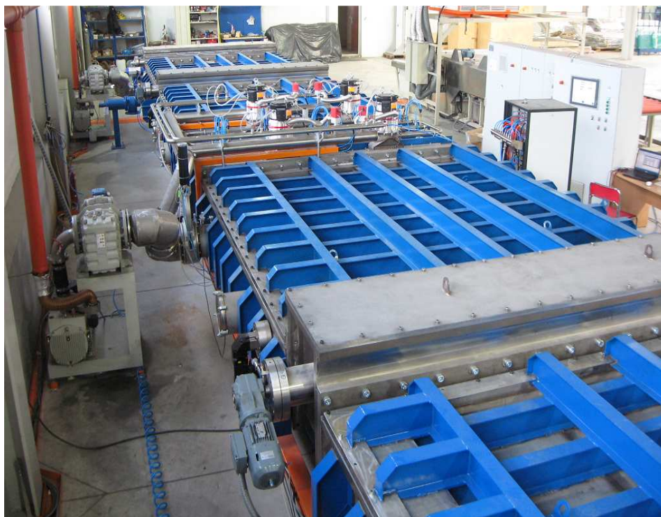
Fig. 2. General view of the line for thin film deposition on glass panels
