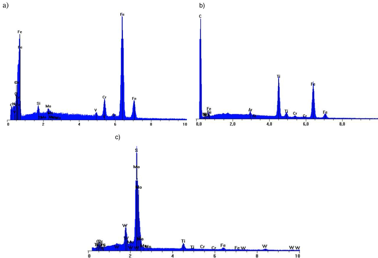
Fig. 4. EDS investigation results of X38CrMoV 5-1 steel samples: a) without PVD coating, b) with TiC+a-C:H coating, c) with MoS<sub>2</sub>TiW coating
