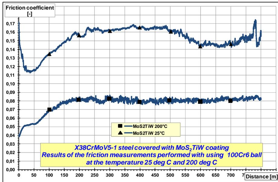
Fig. 7. Comparison of results of friction coefficient measurements of X38CrMoV5-1 steel with MoS<sub>2</sub>TiW coating at the temperature 25 and 200°C performed with using 100Cr6 ball
