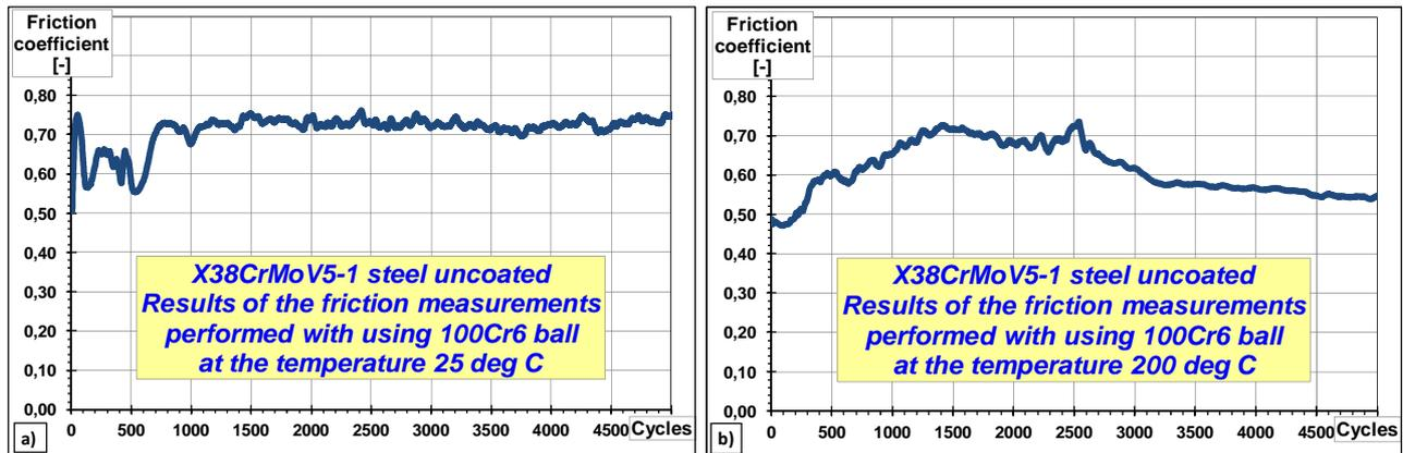
Fig. 5. Friction measurements of X38CrMoV5-1 steel uncoated: a) at the temperature 25°C; b) at the temperature 200°C
