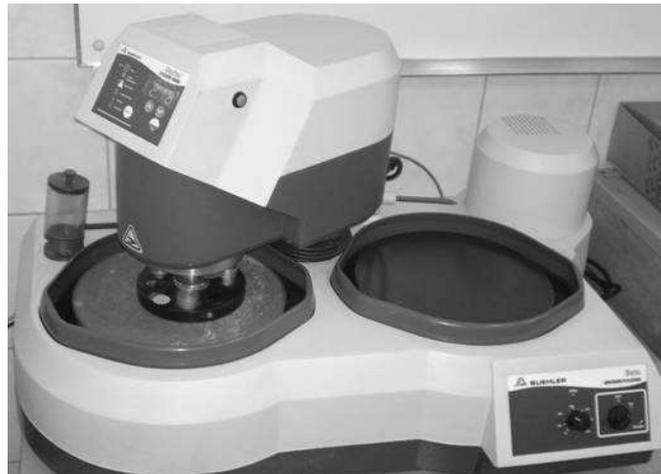
Fig. 2. The overall view of the Beta 2 dual platen grinder-polisher machine equipped with Vector power head and specimens holder
