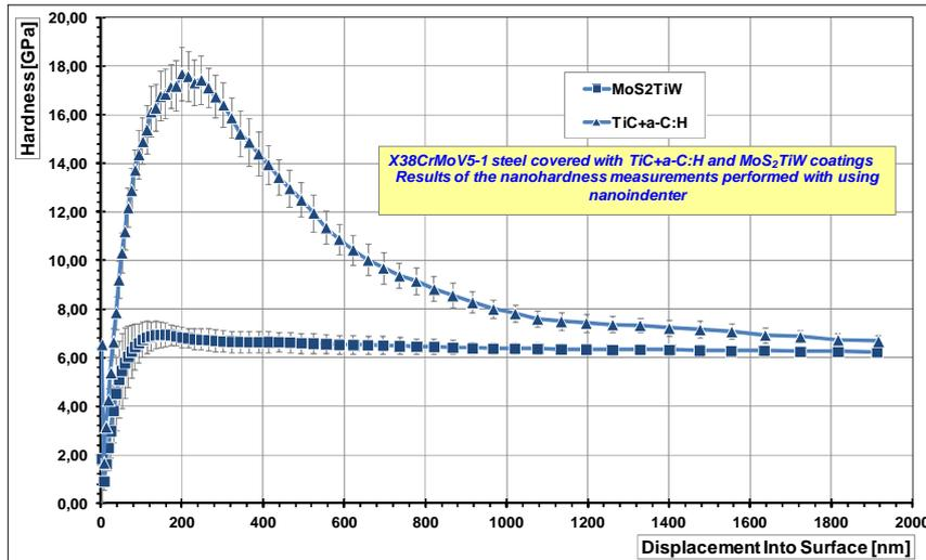
Fig. 8. A comparison of nanohardness measurements of X38CrMoV5-1 steel with TiC+a-C:H and MoS<sub>2</sub>TiW coatings
