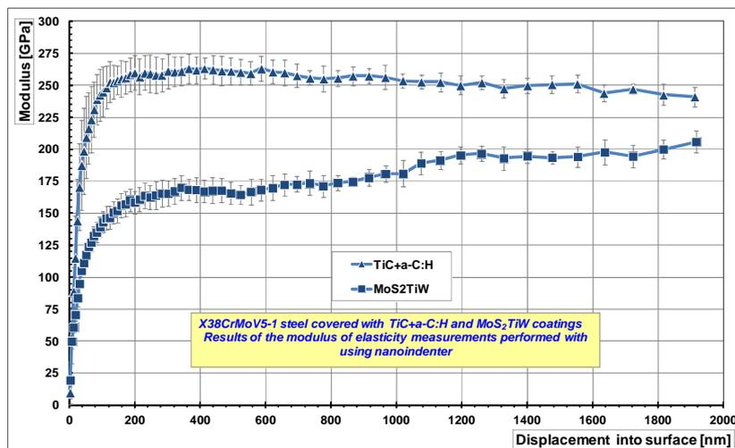
Fig. 9. A comparison of longitudinal modulus of elasticity measurements of X38CrMoV5-1 steel with TiC+a-C:H and MoS<sub>2</sub>TiW coatings
