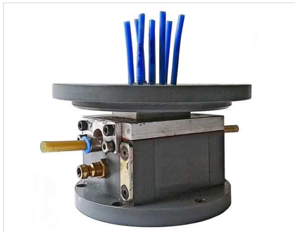
Fig. 1. Machining unit adapted to measuring SM pressure
