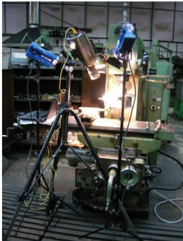
Fig. 3. Research arrangement used to determine the characteristics of the rotational speed of the head drive unit spindle
