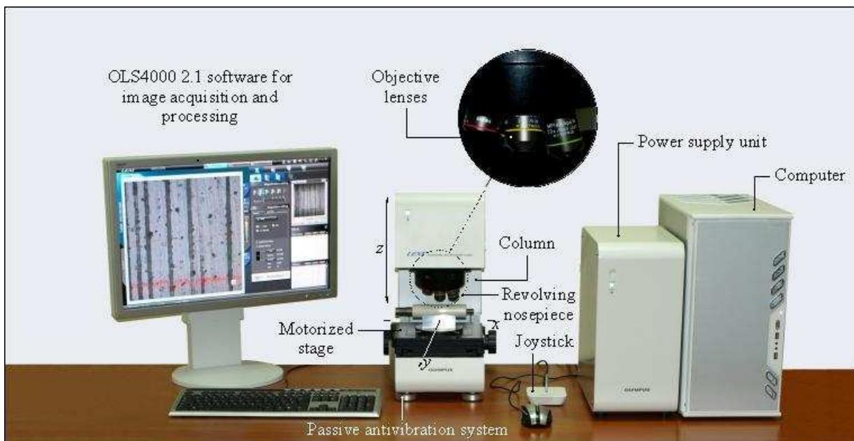
Fig. 5. General view of 3D laser microscope LEXT OLS4000 produced by Olympus
