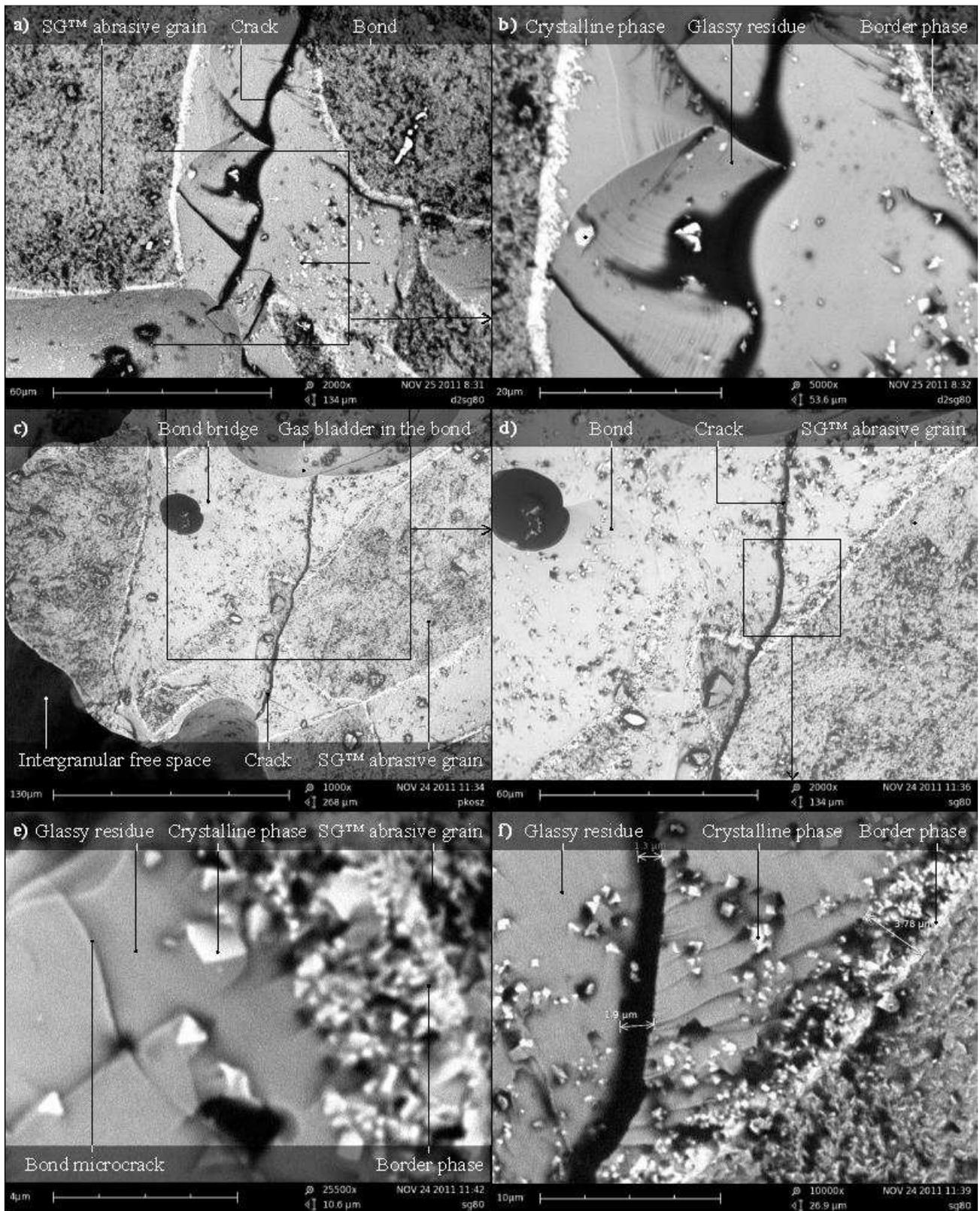
Fig. 11. Collection of selected results of experimental investigations carried out on the breakthrough of the GWAS type 1-35×10×10-SG/F46G10VDG obtained by using of Phenom™ G2 Pro produced by Phenom-World: a) mag. 2000×, b) mag. 5000×, c) mag. 1000×, d) mag. 2000×, e) mag. 25500×, f) mag. 10000×
