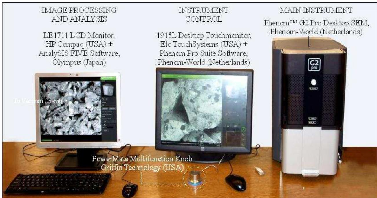
Fig. 9. General view of desktop scanning electron microscope Phenom G2 produced by Phenom-World
