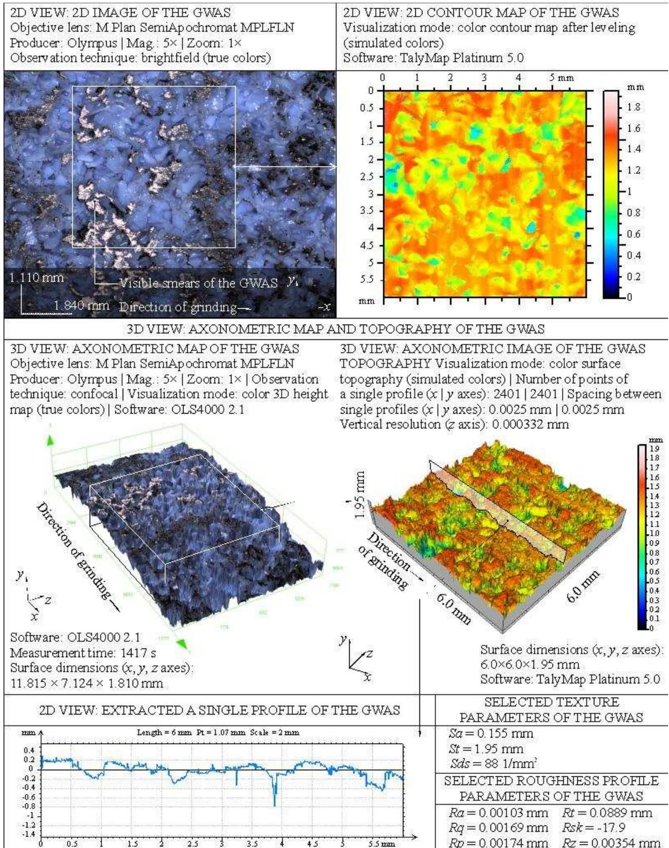
Fig. 7. Collection of selected results of experimental investigations carried out on the GWAS type 1-35×10×10-SG/F46N7VDG by using of 3D laser microscope LEXT OLS4000 produced by Olympus
