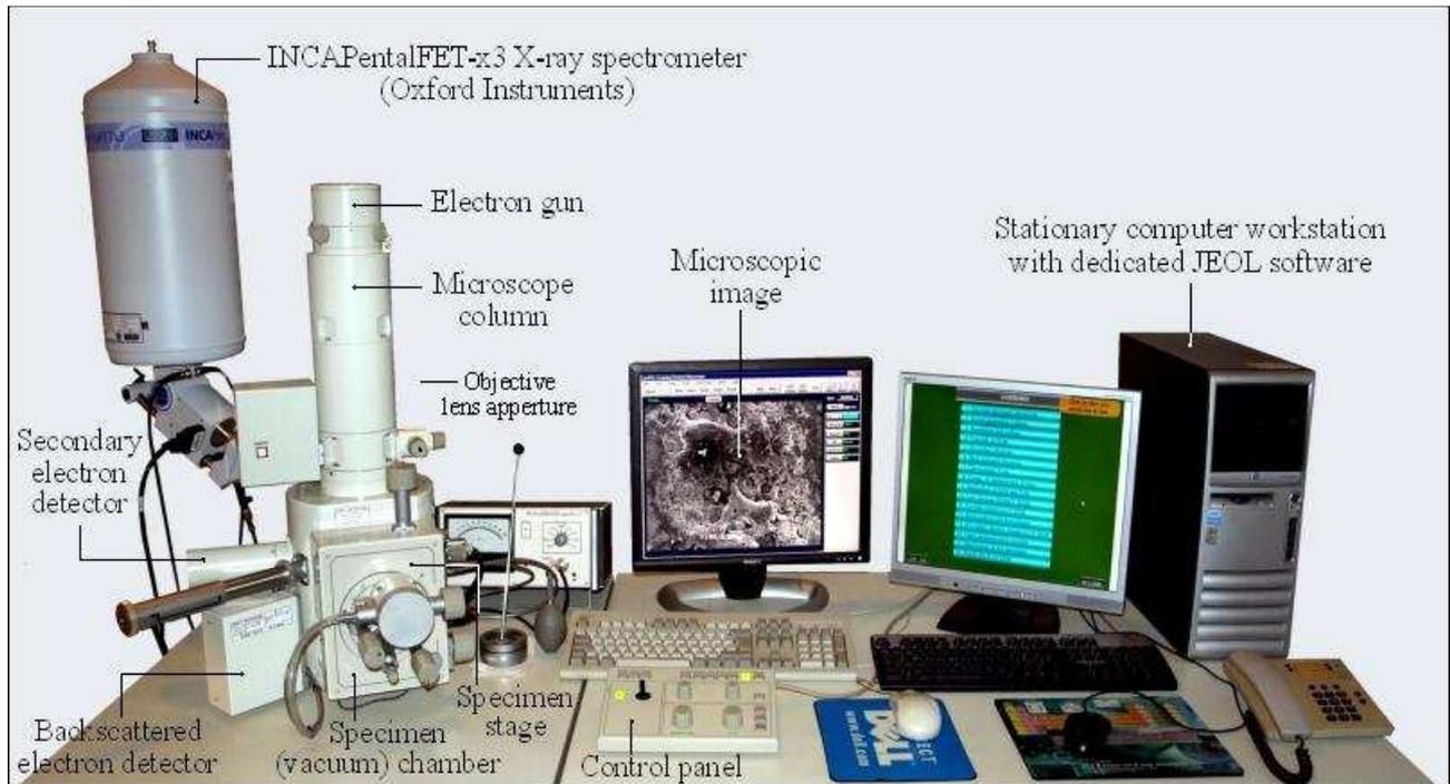
Fig. 8. General view of scanning electron microscope JSM-550LV produced by JEOL
