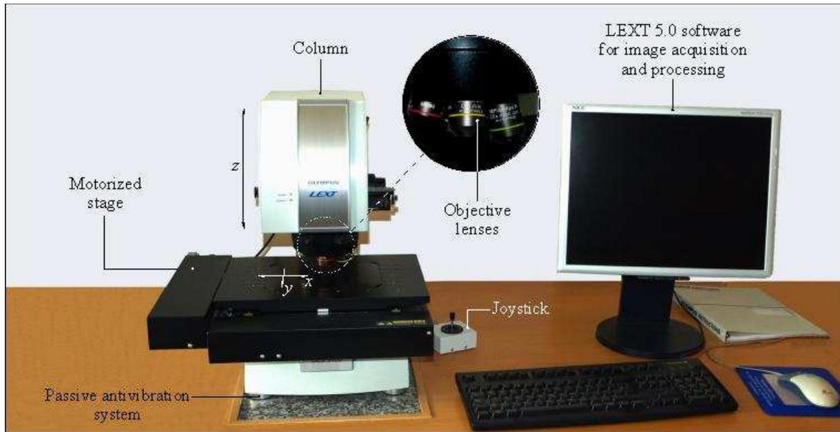
Fig. 4. General view of 3D laser microscope LEXT OLS3100 produced by Olympus
