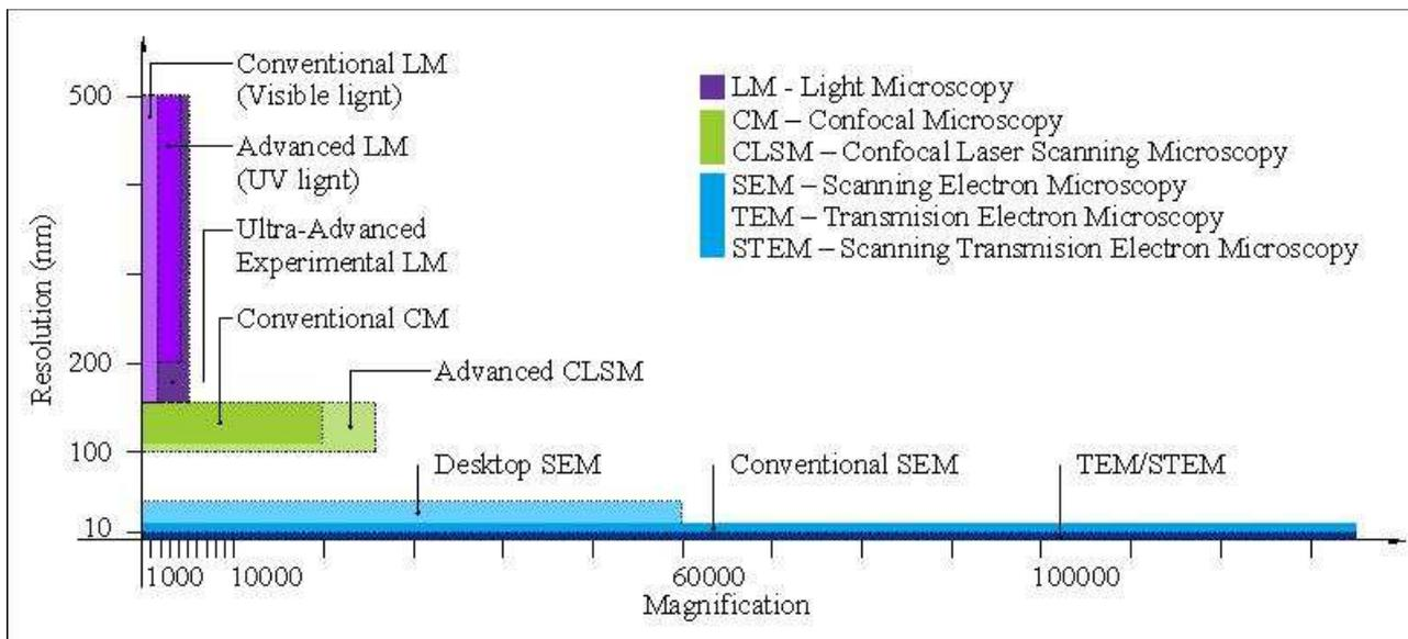
Fig. 1. Classification of selected microscopic techniques in relation to the obtained magnifications and resolutions
