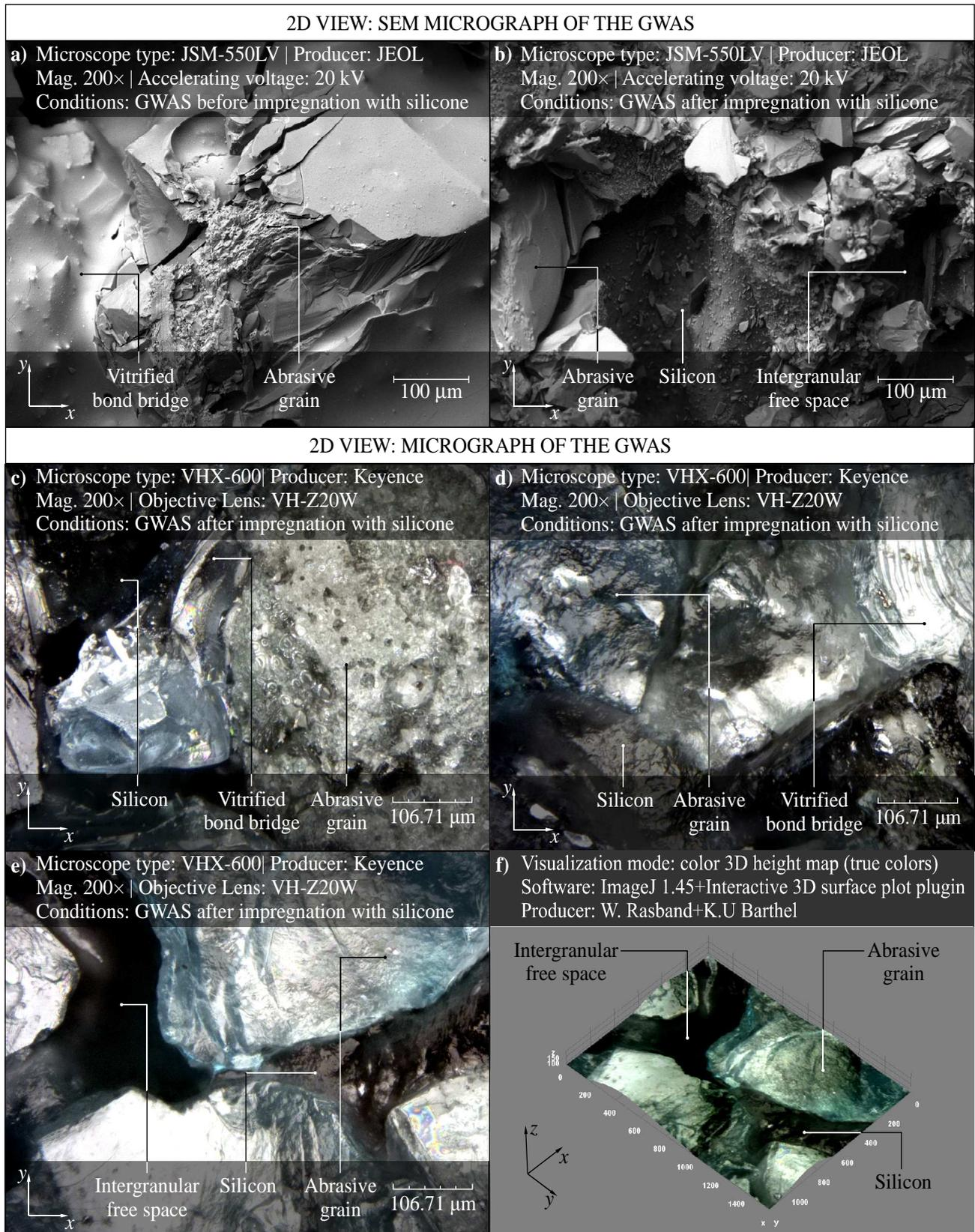
Fig. 3. Collection of selected results of experimental tests carried out on the GWAS type 1-35×10×10-SG/F46 G10VTO by using of: a), b) SEM microscope JSM-550 LV produced by JEOL, c)-e) digital microscope VHX-600 produced by Keyence, f) Image J 1.45 software using interactive 3D surface plot plugin
