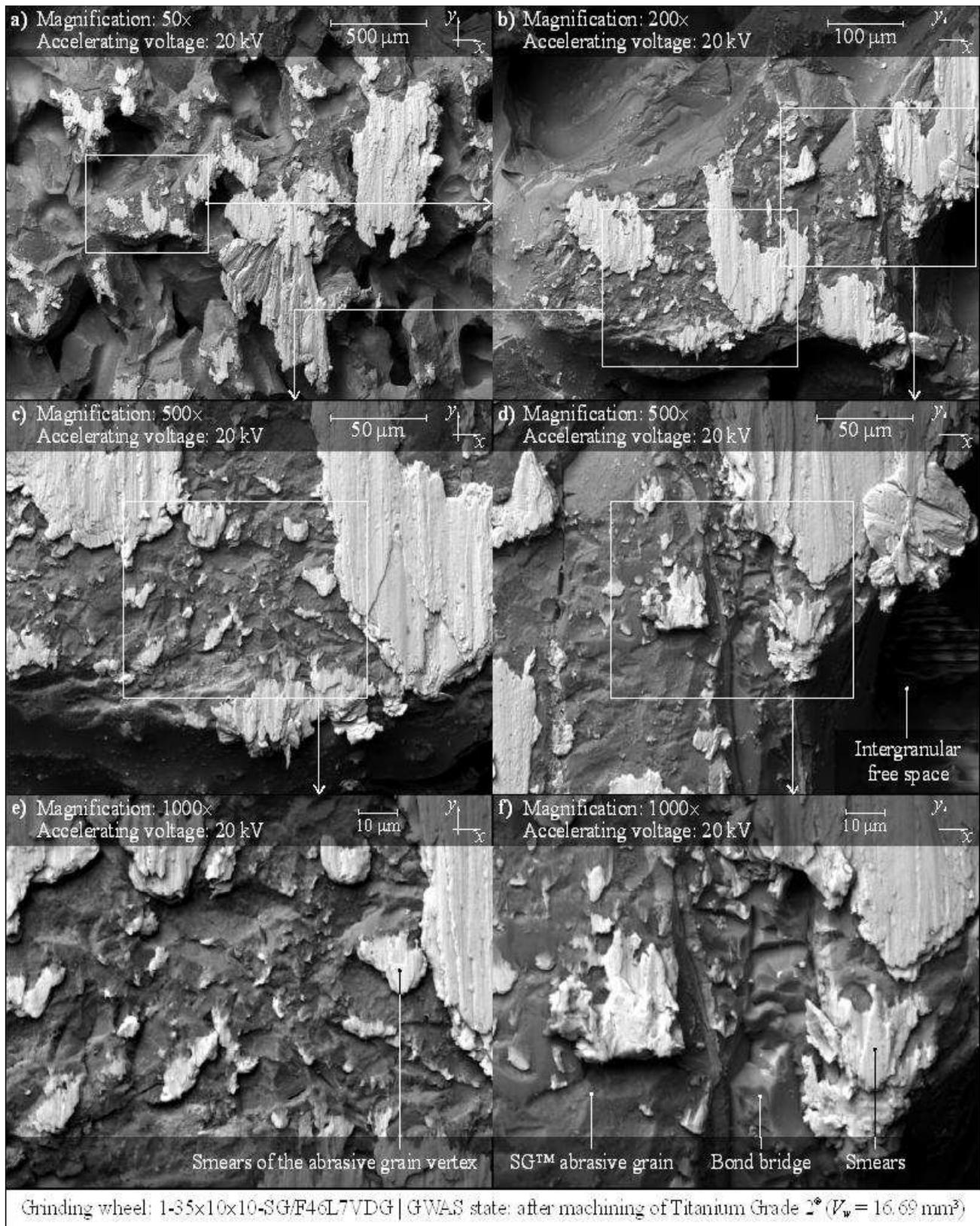
Fig. 10. Collection of selected results of experimental investigations carried out on the GWAS type 1-35×10×10-SG/F46L7VDG after machining process of Titanium Grade 2<sup>®</sup> alloy obtained by using of JSM-550LV produced by JEOL:
