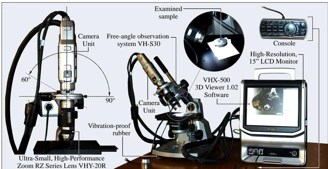
Fig. 2. General view and construction details of digital microscope VHX-600 produced by Keyence
