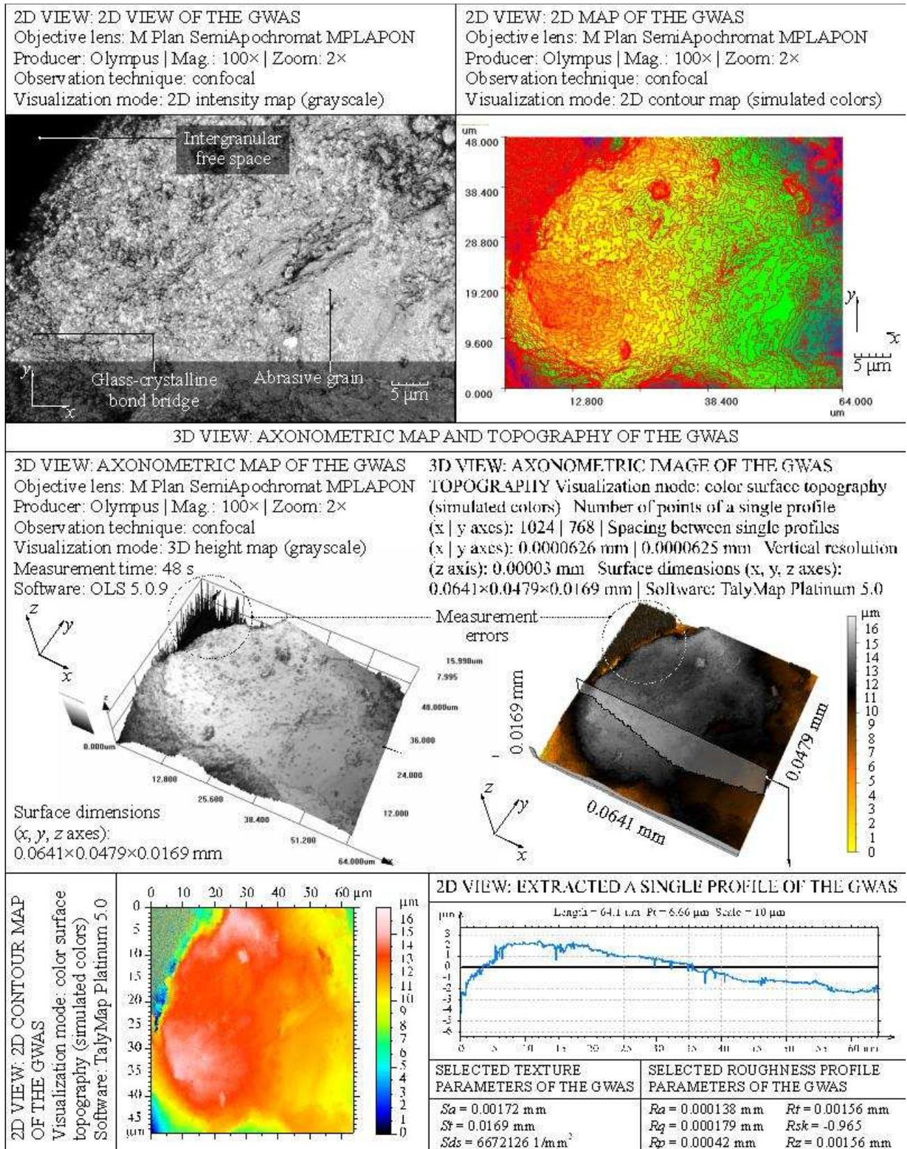
Fig. 6. Collection of selected results of experimental investigations carried out on the GWAS type 1-35×10×10-SG/F46G10VTO by using of 3D laser microscope LEXT OLS3100 produced by Olympus
