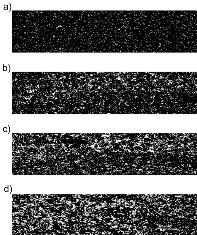
Fig. 4. Results of the detection of flat areas (white) on the abrasive tool's surface: a) the tool before the machining, b) after removing  $2880\text{mm}^3$ , c)  $5760\text{mm}^3$ , and d)  $8640\text{mm}^3$ .
