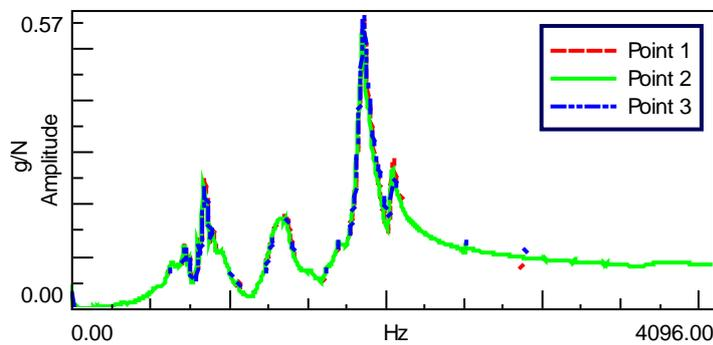
Fig. 3. Acceleration FRFs for points 1, 2, 3 on the workpiece, with VEM, high pre-stress configuration
