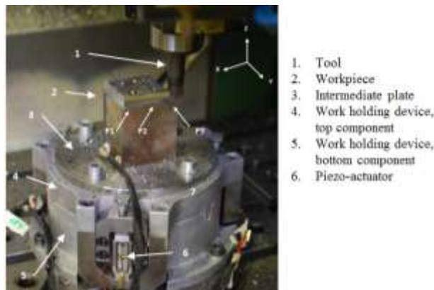
Fig. 1. The experimental setup during machining operation
