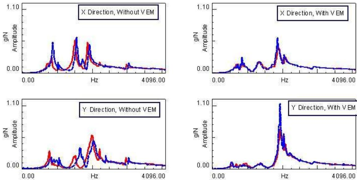
Fig. 2. Comparison of acceleration FRFs for point 1 on the workpiece, red solid lines represent low pre-stress, dashed blue lines represent high pre-stress
