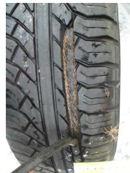
Fig. 7. Circumferential cut with single stream
