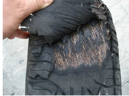
Fig. 9. Result of impact of single stream on flat spread tyre
