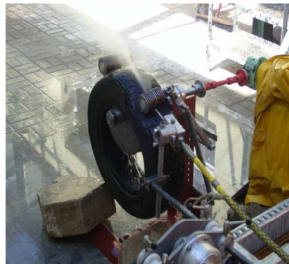
Fig. 5. First attempts of water impact on tyre with various systems of tyre drive
