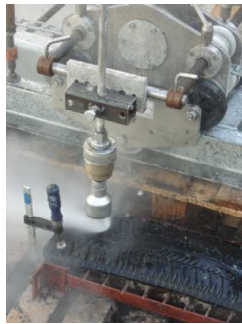
Fig. 10. Cut with head with 3 nozzles on flat tyre
