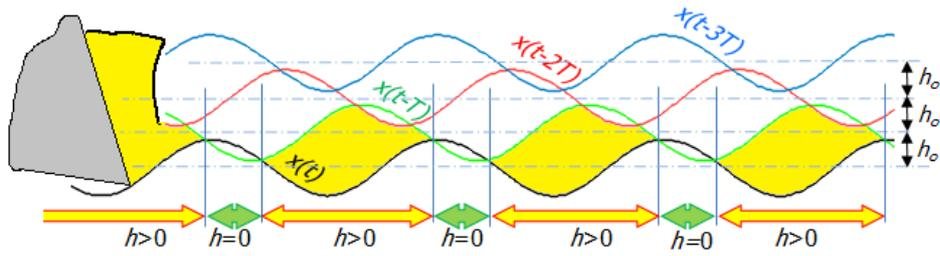
Fig. 6. Exact kinematics approach for surface updating:  $h > 0$  - tool in cut, regular cutting and  $h = 0$  tool out of cut due to excessive vibrations [18]
