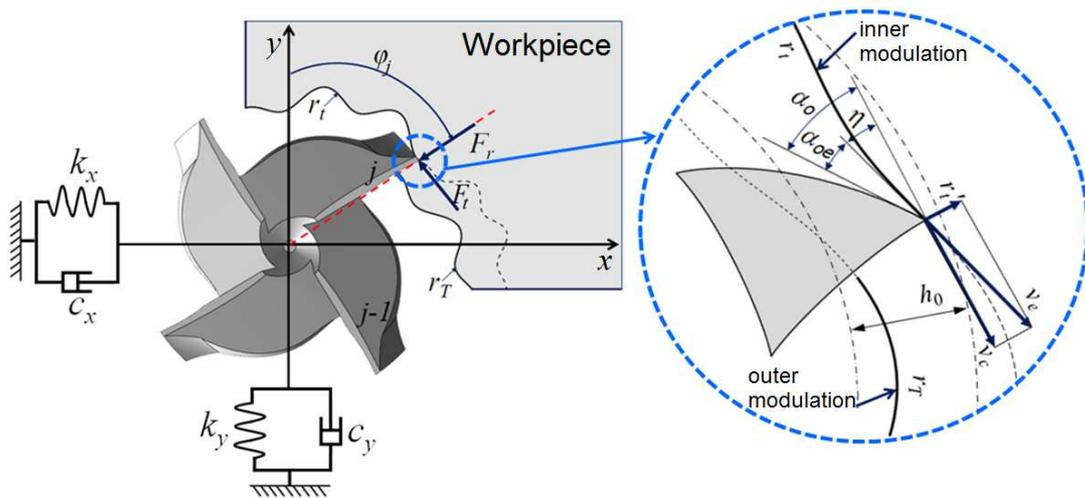
Fig. 1. Dynamic model of 2-DOF system in milling
