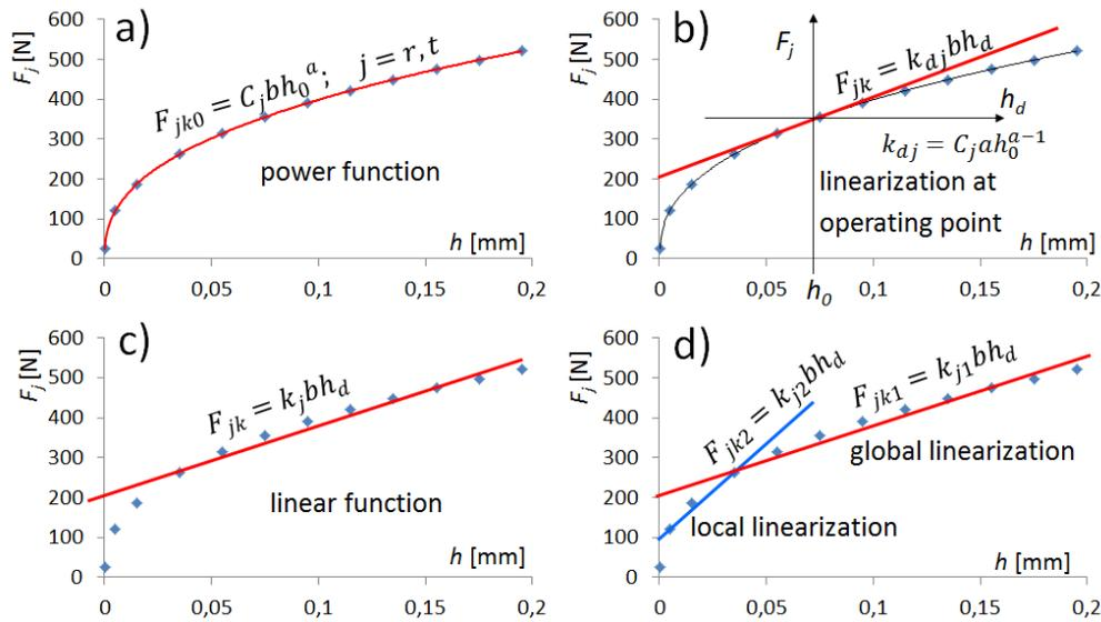
Fig. 7. Dependence of cutting force on the uncut chip thickness: a) non-linear power function, b) linearization at the operating point, c) linear function, d) local and global linearization
