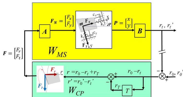
Fig. 2. Block diagram of dynamic 2-DOF system
