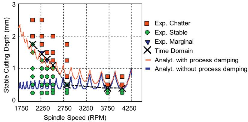
Fig. 8. Comparison of the stability limit obtained experimentally, by time domain simulation, with analytical solution with process damping and without it [8]
