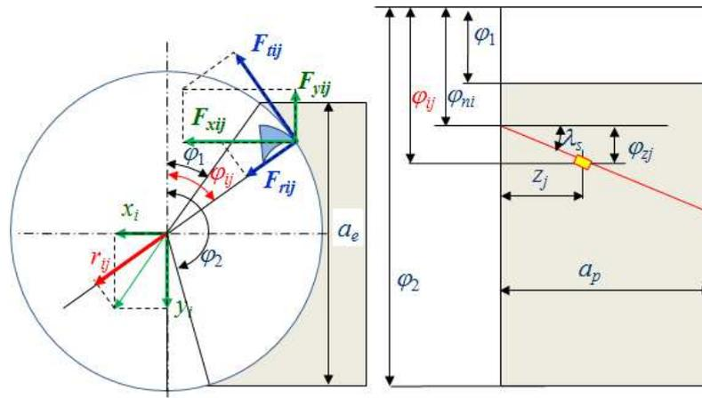
Fig. 4. Discretization of the cutting edge and the distribution of cutting forces for helical flute cutter
