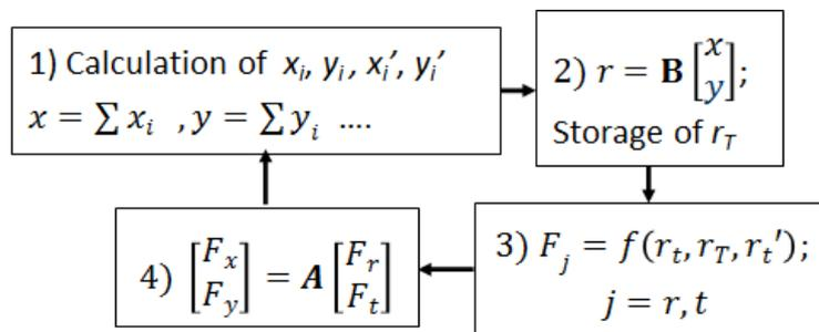
Fig. 3. A single iteration algorithm of numerical simulation of self-excited vibrations
