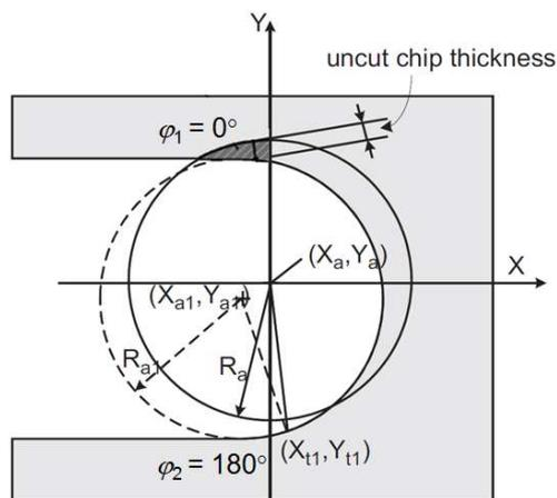
Fig. 5. Backside cutting effect for unstable cutting [22]
