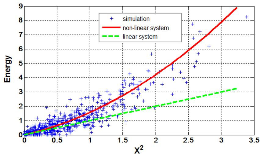
Fig. 5. Kinetic  $1/2 \dot{x}^2$  and potential  $U(x)$  energy for a heavier damped system, 1%
