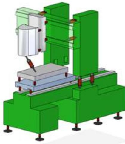
Fig. 2. Machine tool with represented joints [4]
