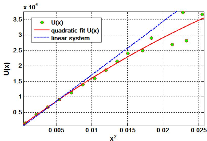
Fig. 14. Stiffness estimation - stable machining
