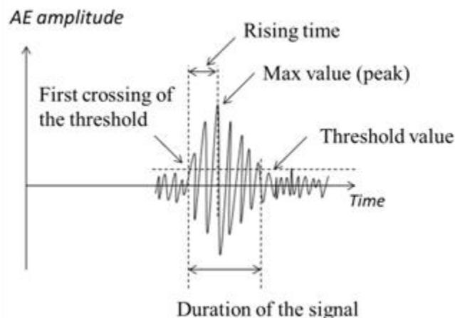
Fig. 1. The basic features of a “burst” type acoustic emission event
