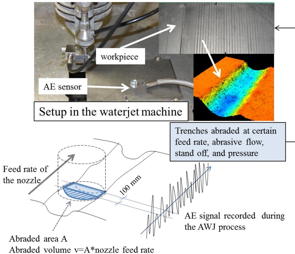
Fig. 2. Experiment arrangement. Abraded trench and AE recorded during the AWJ machining
