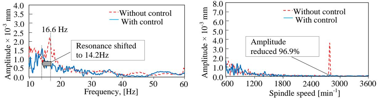
(a). Frequency response by impact test (Right) and vibration amplitude operated at 2784min<sup>-1</sup> (Left) in X-axis
