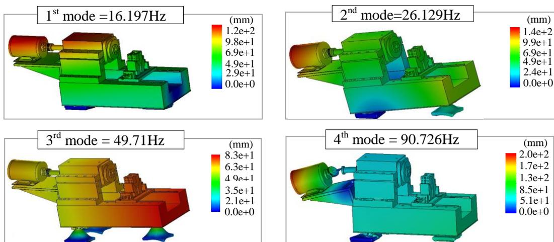
Fig. 1. Simulation results of mode shapes of bench lathe at free vibration studied using CosmosWorks software
