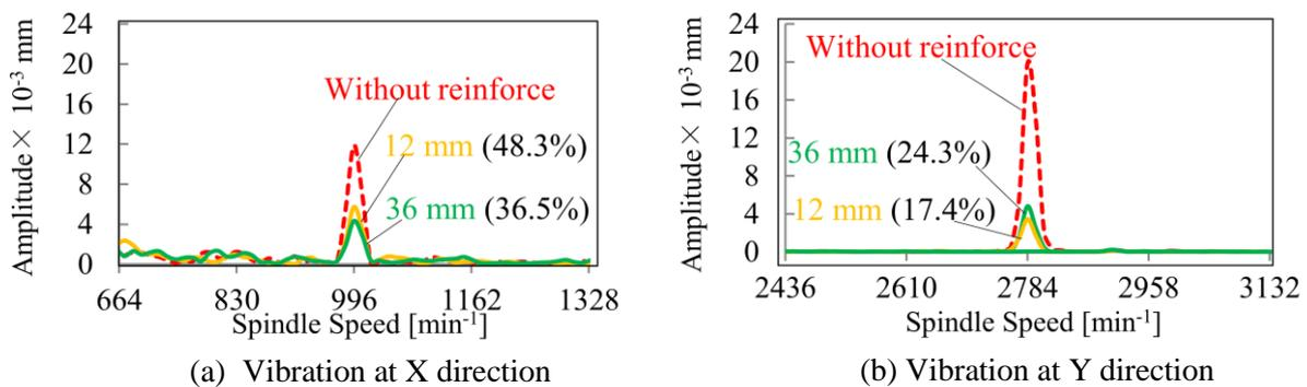
Fig. 11. Relationship between the spindle speeds at machine resonance with the amplitude of vibration by using reinforce frame
