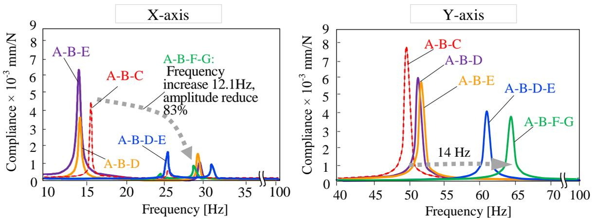
Fig. 5. Frequency response of the bench lathe from X-axis and Y-axis with different support positions
