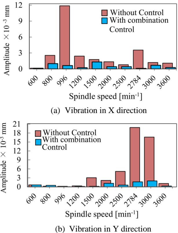
Fig. 13. Amplitude of vibration using three combination control (Experimental results)
