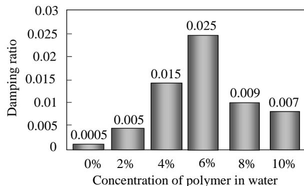
Fig. 7. The relationship between polymer percentage and the damping ratio
