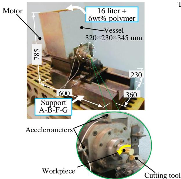
Fig. 14. Photograph of experimental setup for real cutting
