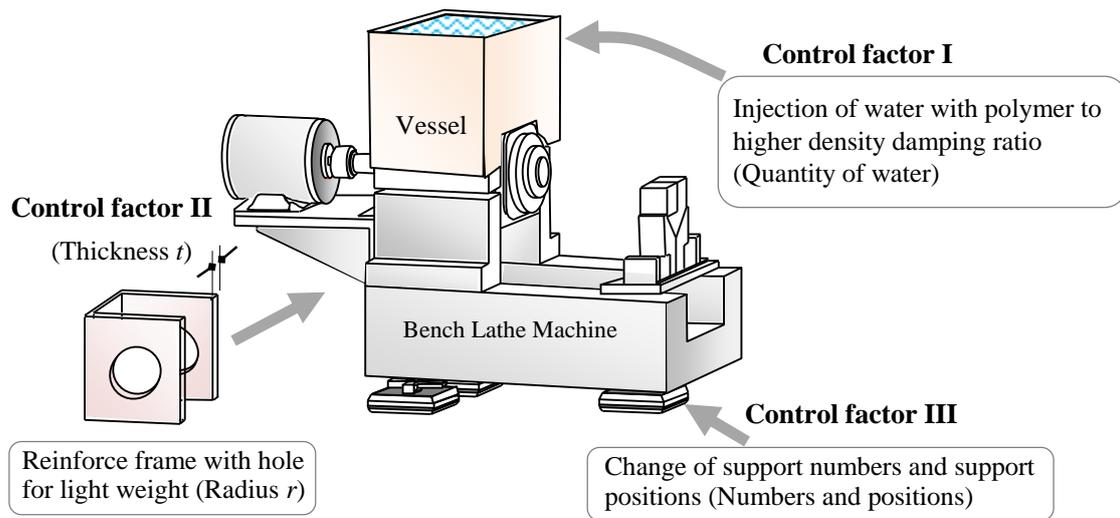
Fig. 2. Explanation of parameters and countermeasures for controlling resonance in a machine tool
