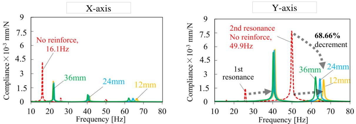
Fig. 4. Frequency response of the bench lathe from X-axis and Y-axis with reinforce motor base
