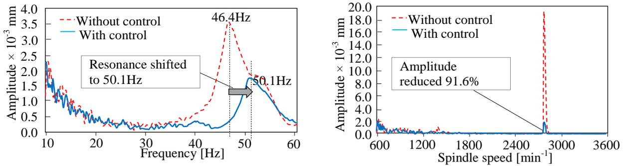
(b). Frequency response by impact test (Right) and vibration amplitude operated at 2784min<sup>-1</sup> (Left) in Y-axis
