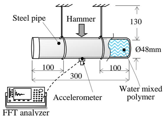
Fig. 6. Experimental setup for measuring damping ratio
