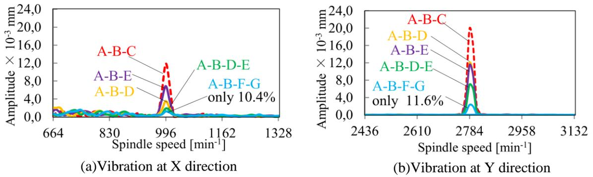
Fig. 12. Relationship between the spindle speeds at machine resonance with the amplitude of vibration by control of support positions
