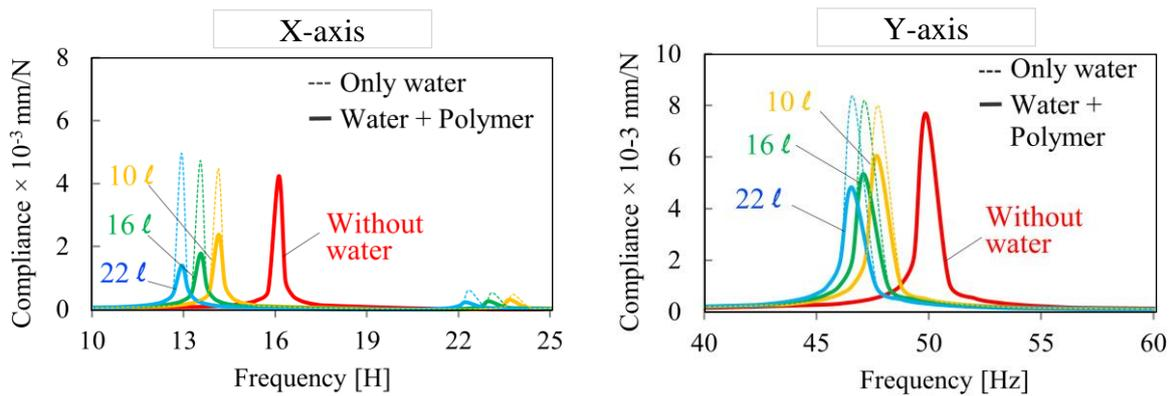
Fig. 8. Comparison of frequency response without polymer and with 6wt% polymer concentration
