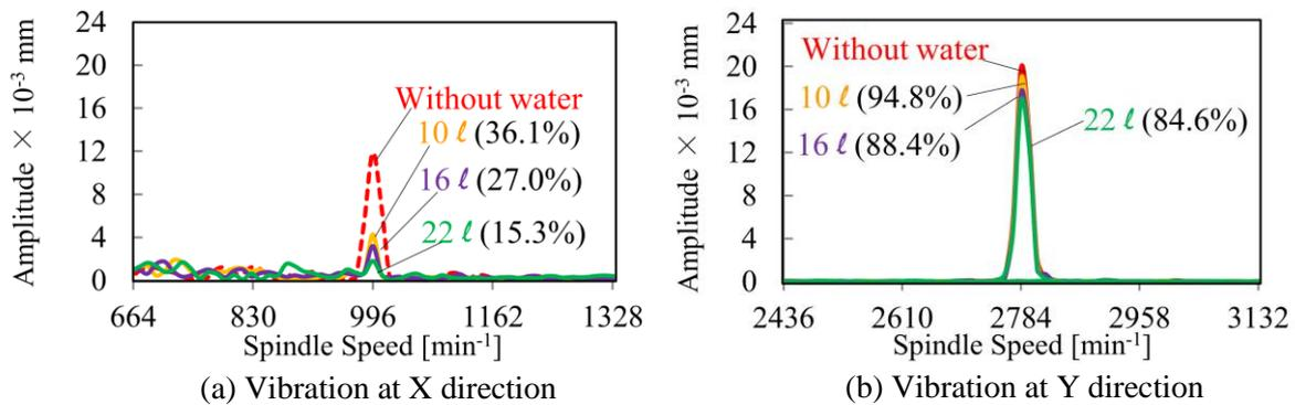
Fig. 10. Relationship between the spindle speeds at machine resonance with the amplitude of vibration by injecting polymer
