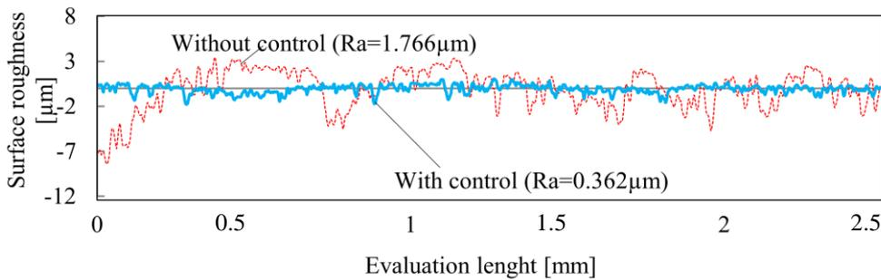
Fig. 16. Comparison of surface roughness after cutting using proposed control technique
