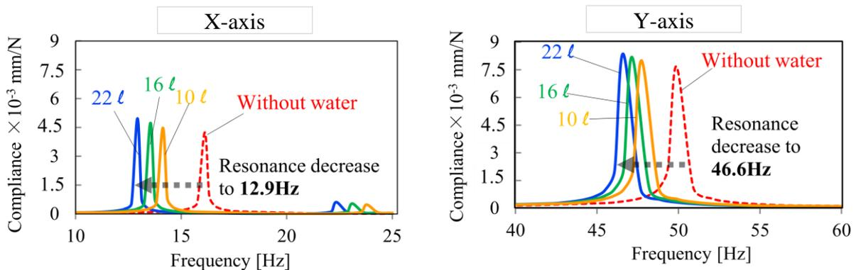
Fig. 3. Frequency response of the bench lathe from X-axis and Y-axis by injecting water
