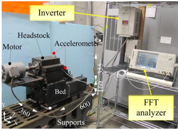
Fig. 9. Experimental set up and the model of bench lathe
