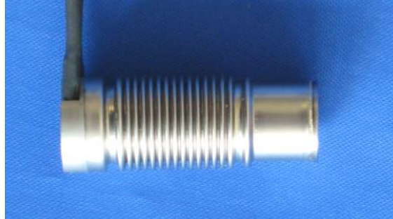
Fig. 5. Custom made piezoelectric ceramics
