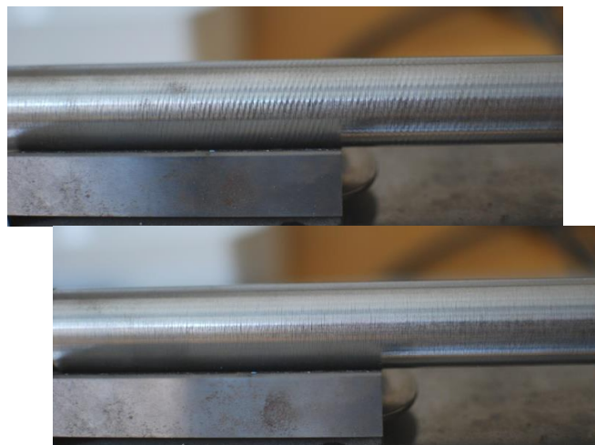
Fig. 14. Appearance of the chatter on the machined bar and machining with semi-active damping system
