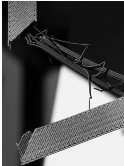
Fig. 8. Fracture in the partially filled ABS samples (sparse distance 11,43mm)
