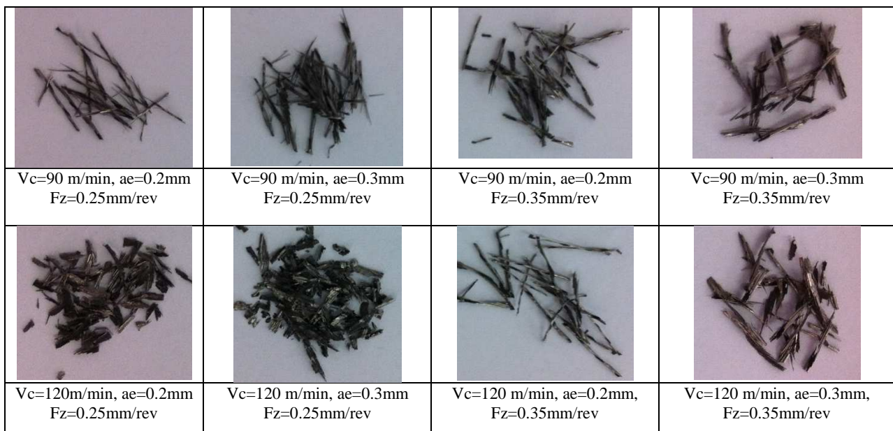
Fig. 7. Chip morphology
