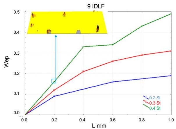
Fig. 9.  $w_{ep}$  index depending on the length of 9IDLF film
