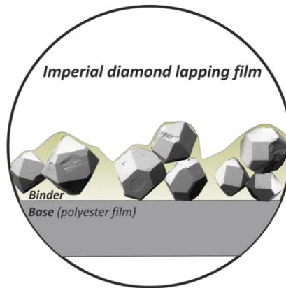
Fig. 2. Structure of diamond abrasive films
