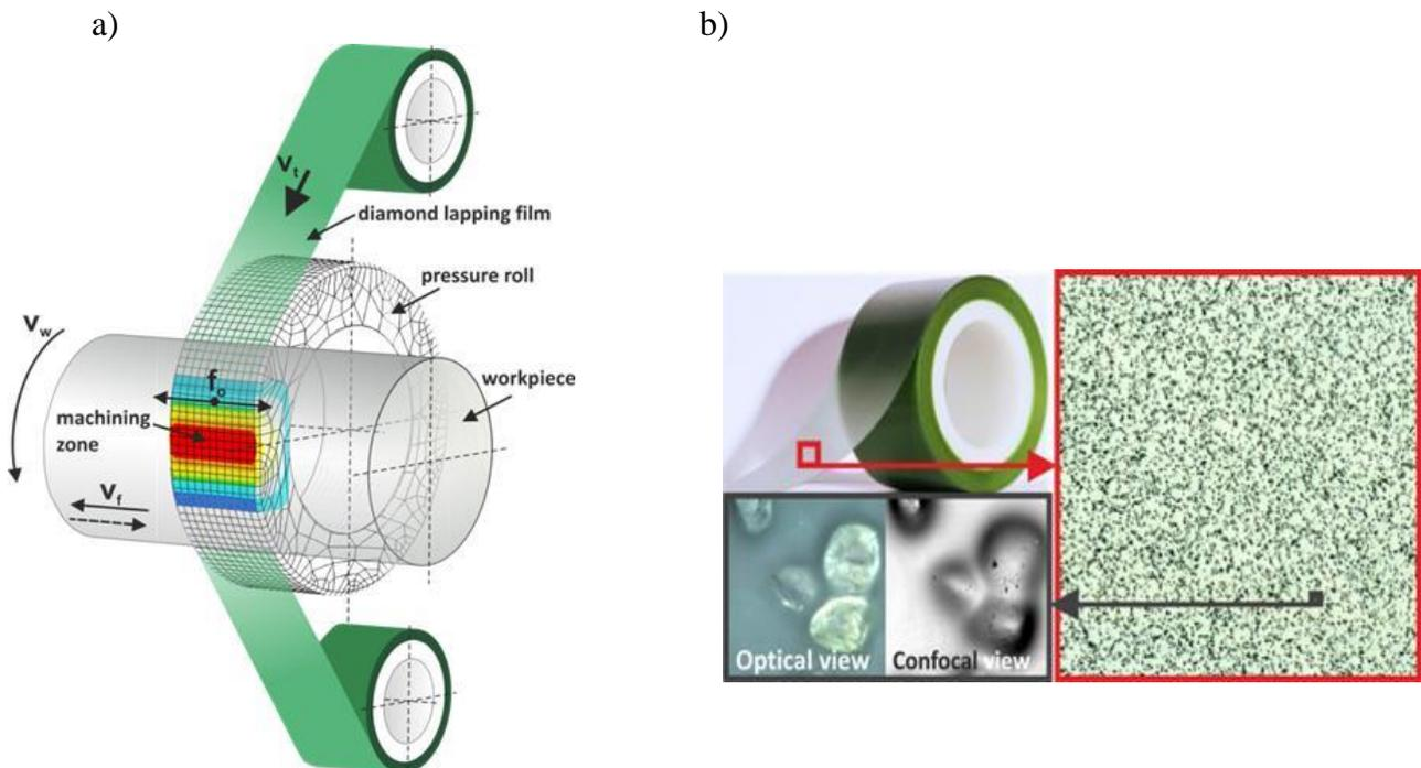
Fig. 1. Machining system for additional finishing of surface (a), where:  $f_o$  – oscillating motion of the tool,  $v_w$  – direction of circular motion of the object,  $v_f$  – direction of feed motion,  $v_l$  – direction of displacement of abrasive grain and (b) roll of abrasive film with visible abrasive grains embedded in glue
