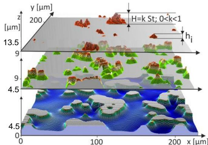
Fig. 5. Scheme for the evaluation of distribution of grains' vertices on the surface of abrasive film exemplified by 9IDLf abrasive grain surface
