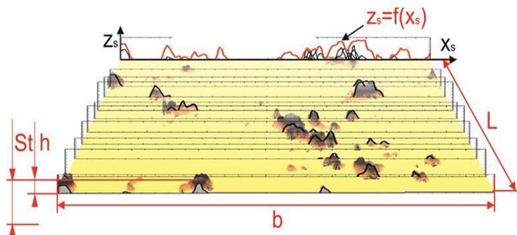
Fig. 6. The overall profile of the film  $z_s = f(x_s)$  in the form of an envelope of sum of projection gradients above  $H$  level, on  $z_s, x_s$  plane
