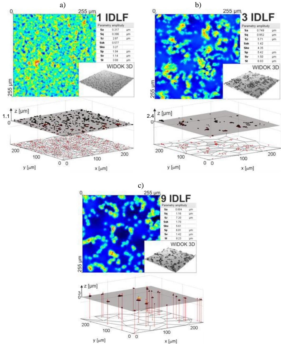
Fig. 4. Heights and surface gradients above the plane distant from the highest vertex by  $H=kSt$  value and representation of surface decomposition on Voronoi cells on the surface of diamond abrasive films of nominal grain size  $a_g$  1 μm (a), 3 μm (b) and 9 μm (c)
