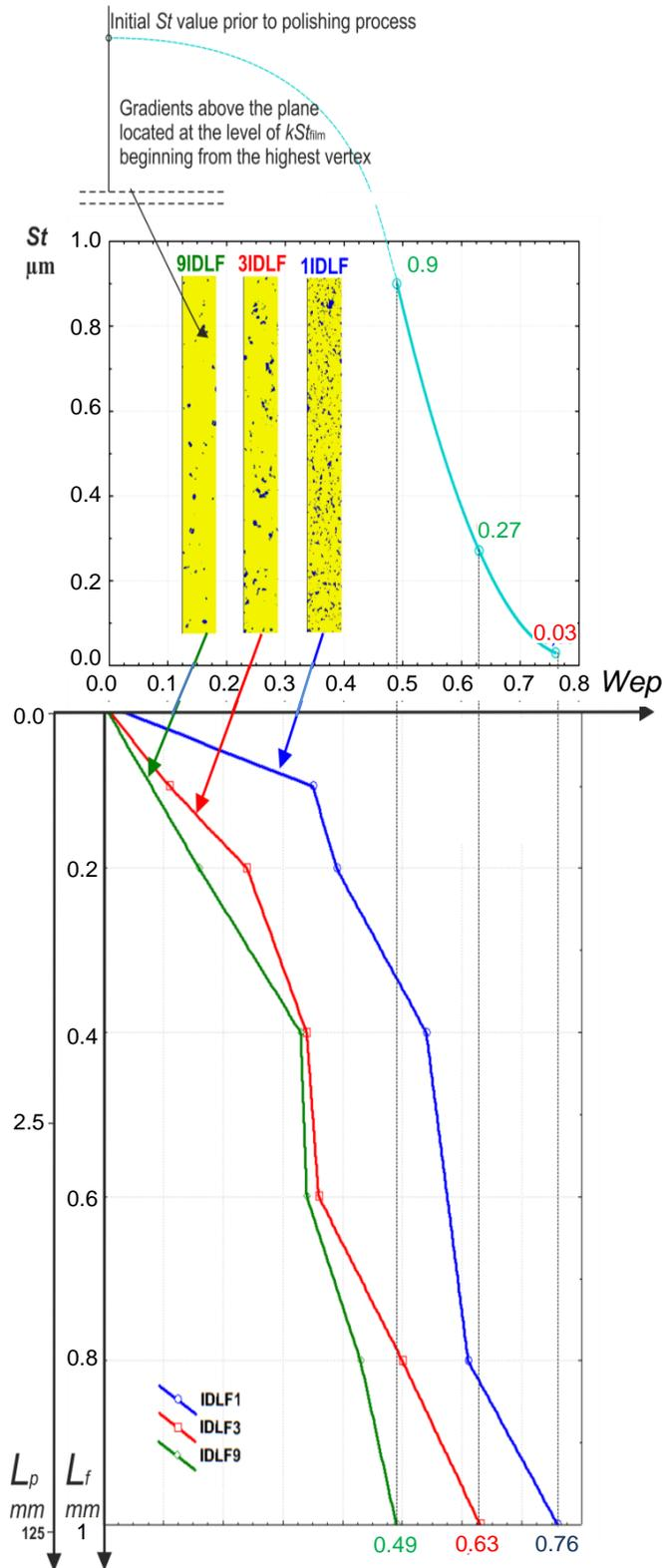
Fig. 10. The relationship between  $St$  parameter of the microfinished surface and the value of  $w_{ep}$  index determined for the plane position  $H=0.4St$ , for the film length  $L_f=1$  mm and the contact length the workpiece  $L_p=125$  mm
