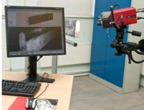
Fig. 1. 3D scanning by ATOS II 400
