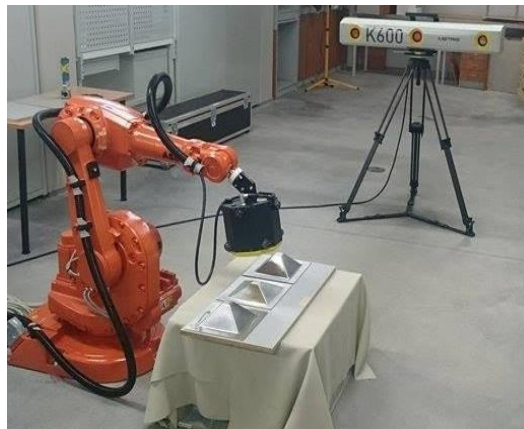
Fig. 2. Scanning by Nikon K-Robot scanning system
