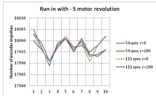
Fig. 6. Dependence of the angle of table rotation on the set angle of motor rotation: set angle of motor rotation: a) 1 revolution; b) 5 revolutions, for two velocity values: 54 and 111 RPM and two ramp values: 0 and 200 impulses, for 10 repetitions [5]
