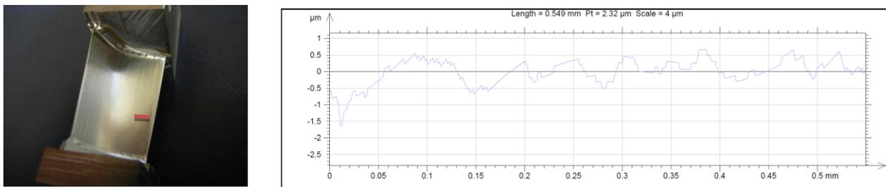
Fig. 16. The example of surface profile measurement of pressure side of the blade milled by NC programs based on TCP function
