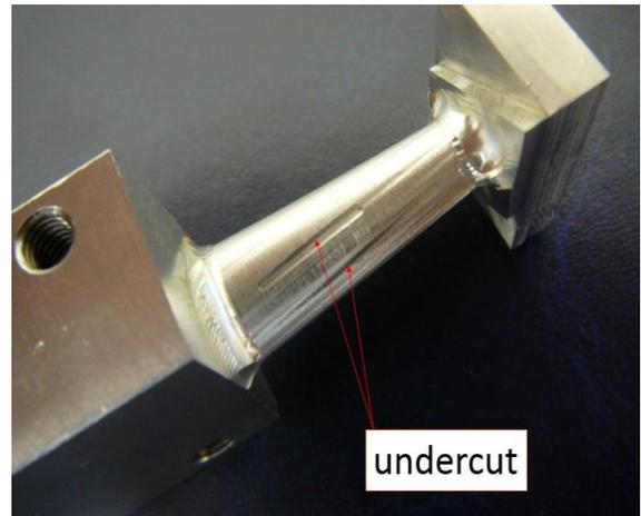
Fig. 9. Consequences of toolpath errors
