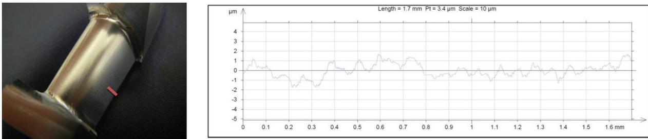
Fig. 15. The example of surface measurement of suction side of the blade milled by NC programs based on TCP function
