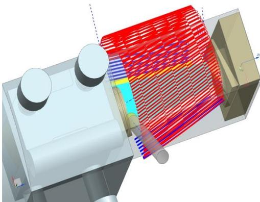
Fig. 10. Suction side finishing
