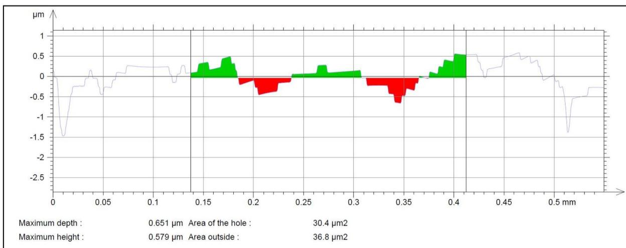
Fig. 14. The measurement of surface profile on the suction surface of the blade in a perpendicular direction to the flow
