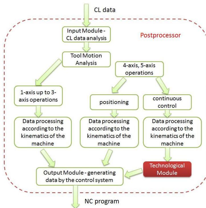
Fig. 2. Schematic location of technological module postprocessor
