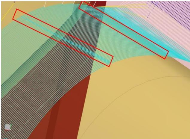
Fig. 8. Toolpath errors (marked by red rectangles)
