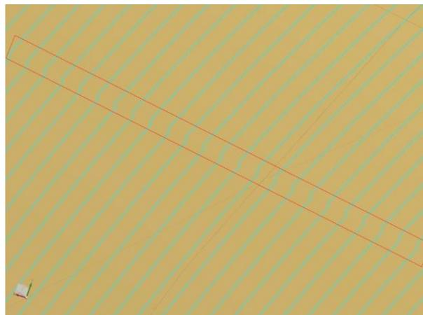
Fig. 13. Toolpath errors (marked by red rectangle)
