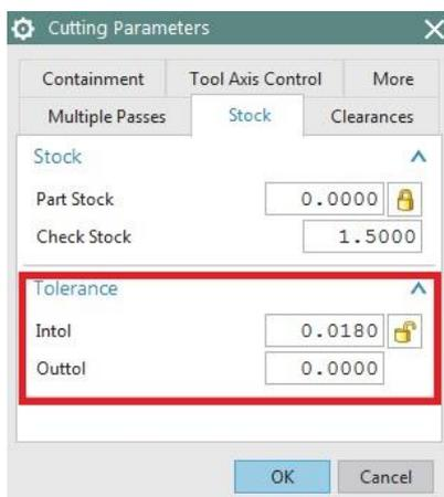
Fig. 12. CAM tolerance setting
