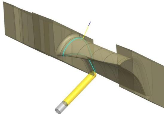
Fig. 5. Testing toolpath on the blade surface
