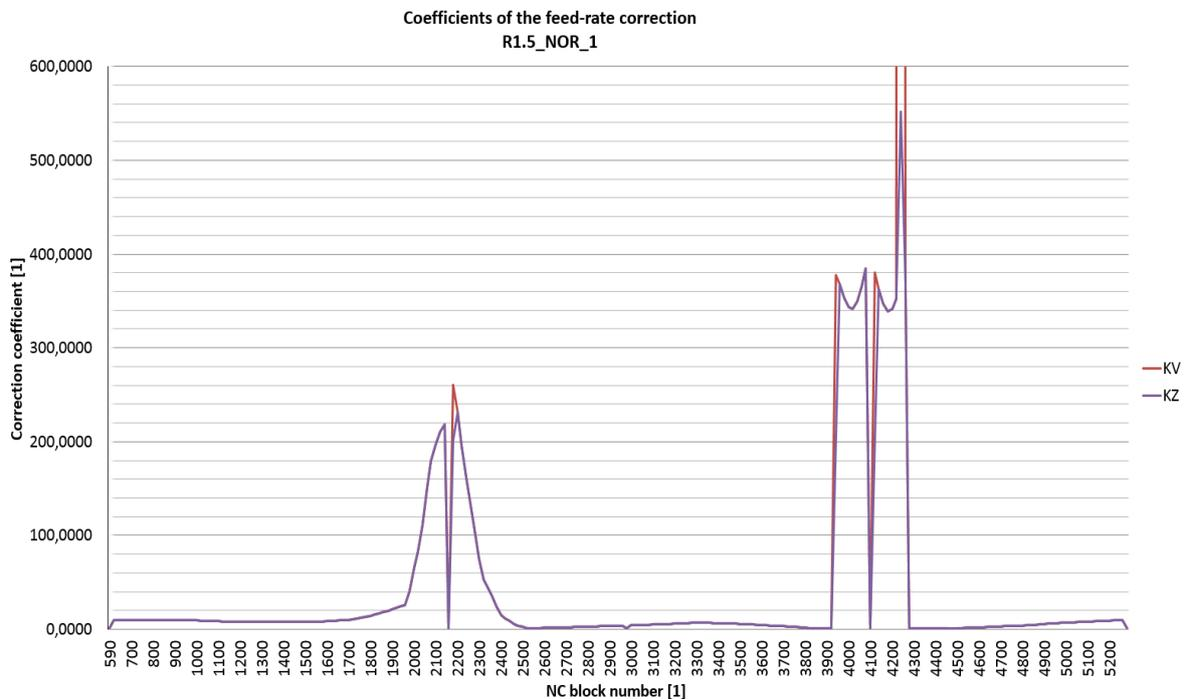
Fig. 7. Comparison of not smoothed (KV) and smoothed (KZ) feed-rate correction coefficient depending on the number of block of the NC program
