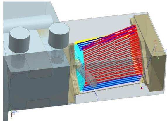
Fig. 11. Pressure side finishing
