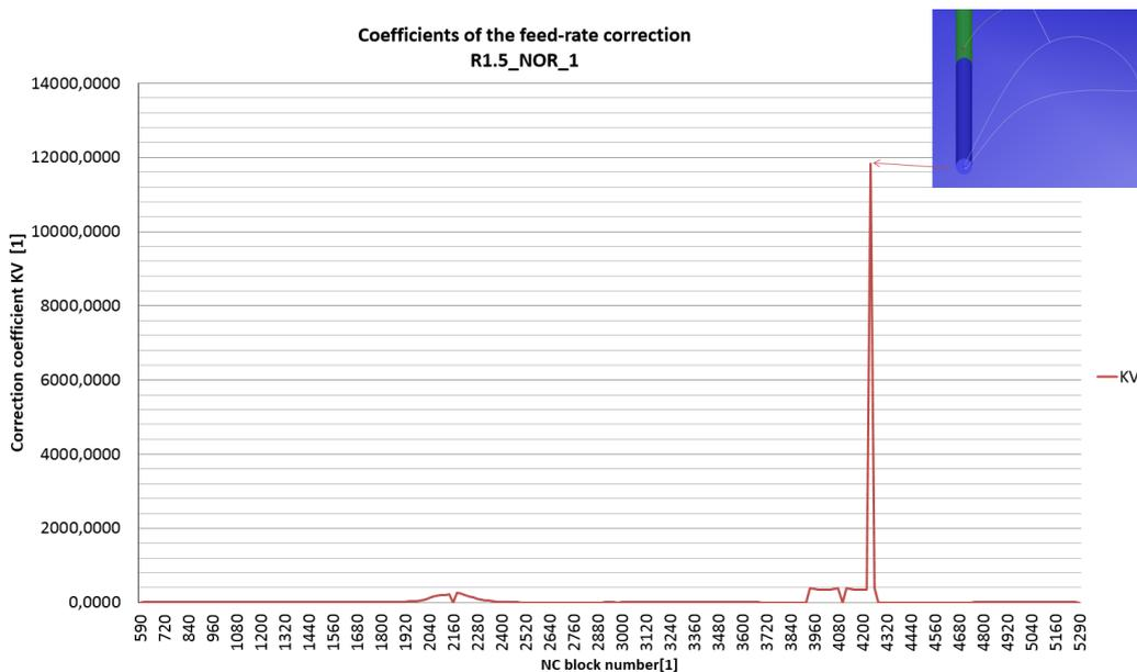
Fig. 6. Graph of the correction coefficient KV according to the block of the NC program
