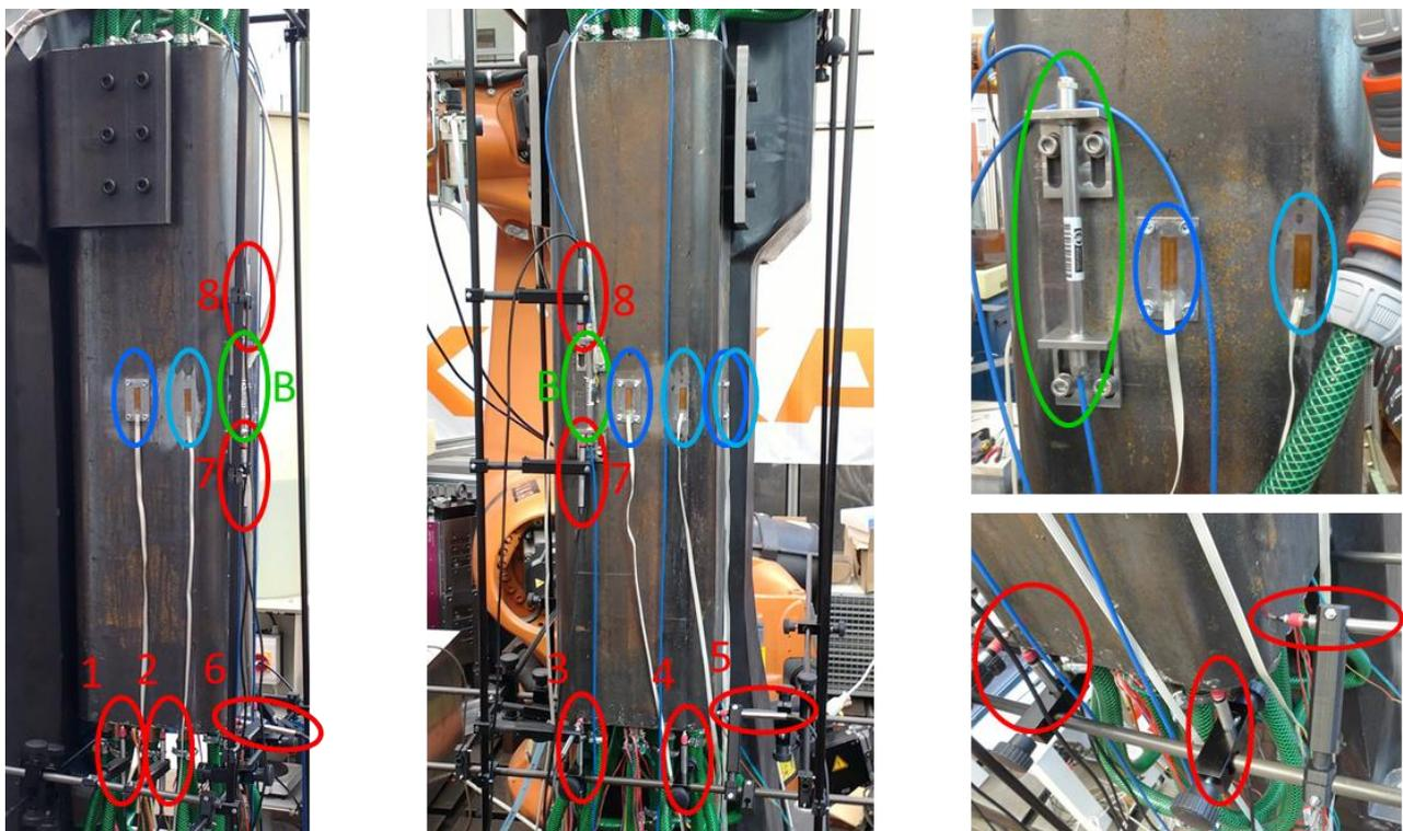
Fig. 4. Arrangement of external strain and displacement sensors (light blue: directly mounted strain gauges, blue: indirectly mounted strain gauges, green: fibre optic Bragg sensor, red: displacement sensors)
