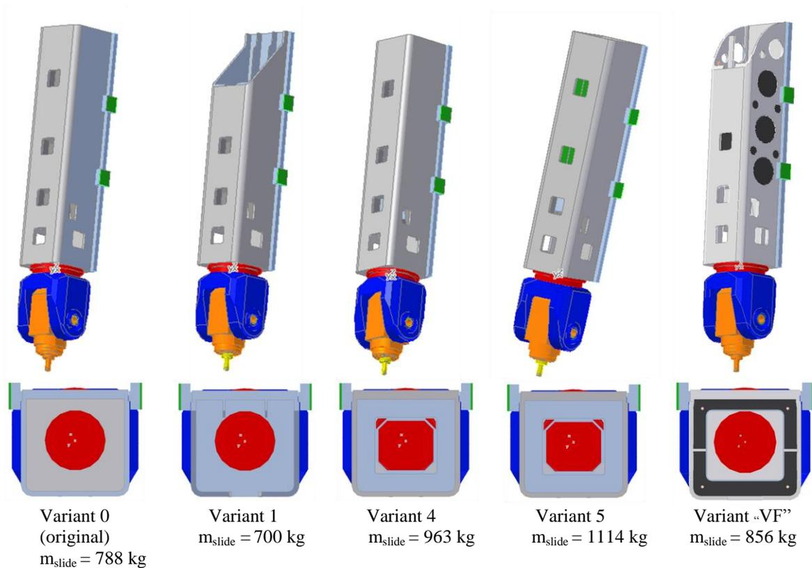
Fig. 9. Selected design variants of the z-slide (position P1)
