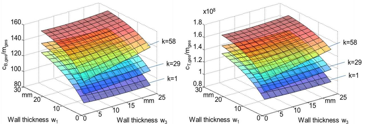
Fig. 8. Specific bending (left) and torsional (right) spring constants of sandwich profile variants
