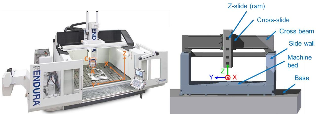
Fig. 1. Exemplary five axis overhead gantry type milling machine ENDURA 700 linear
