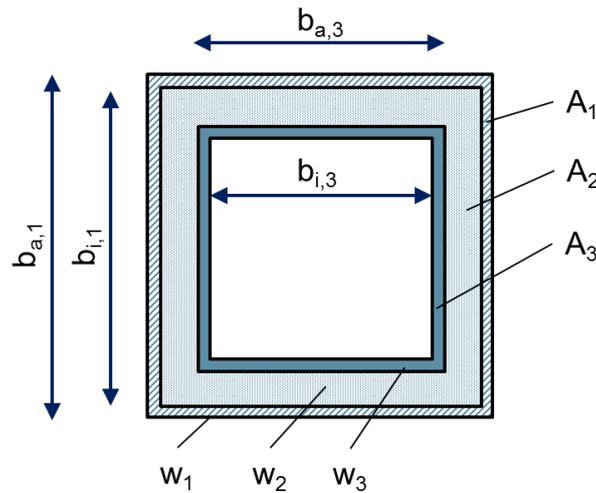
Fig. 7. Cross section of an abstract sandwich type hollow profile with three layers
