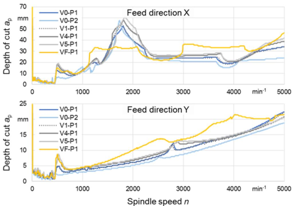
Fig. 11. Stability charts for the slide variants with feed directions in X and Y
