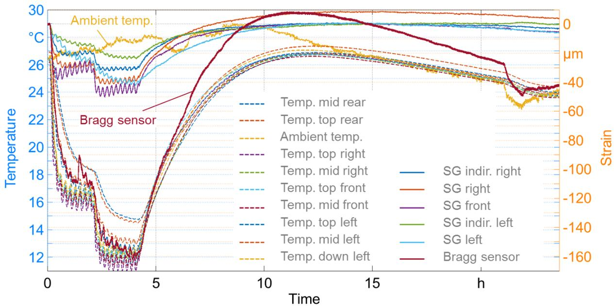
Fig. 5. Results of measurements with active cooling of the hybrid material test component (SG: strain gauge)
