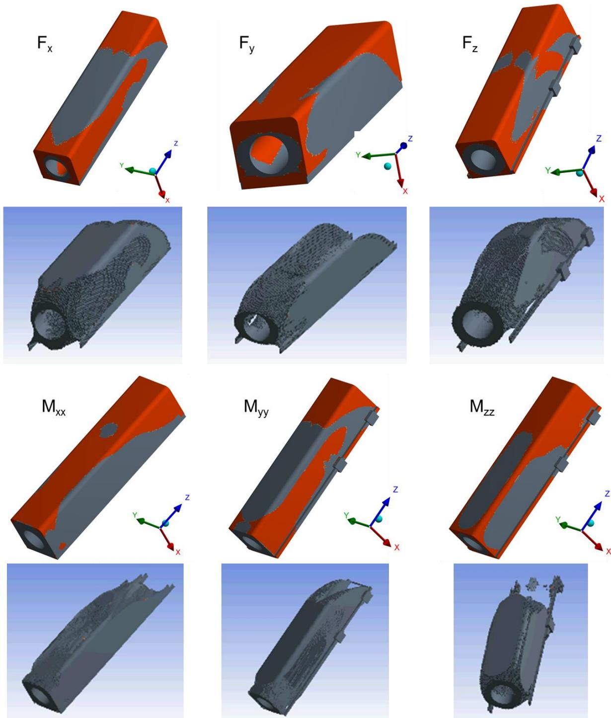
Fig. 6. Topology optimisation of a simplified slide body under various loads
