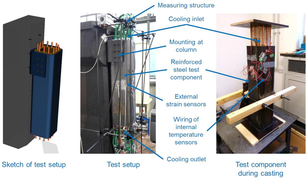
Fig. 3. Test setup for active cooling experiments
