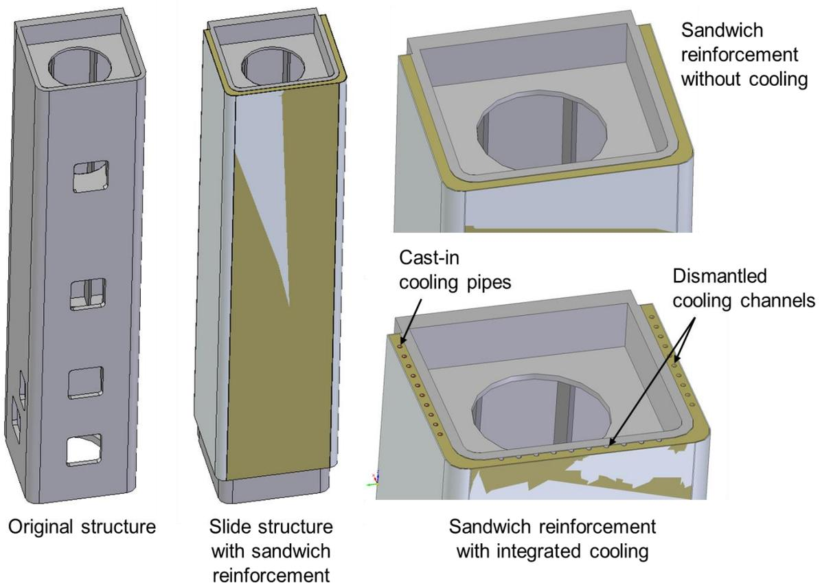
Fig. 2. Principle approach of sandwich reinforcement with integrated active cooling
