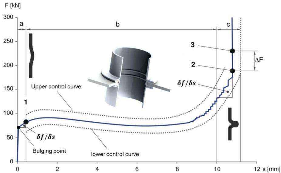
Fig. 4. Force-displacement curve and upset bulging process control strategy
