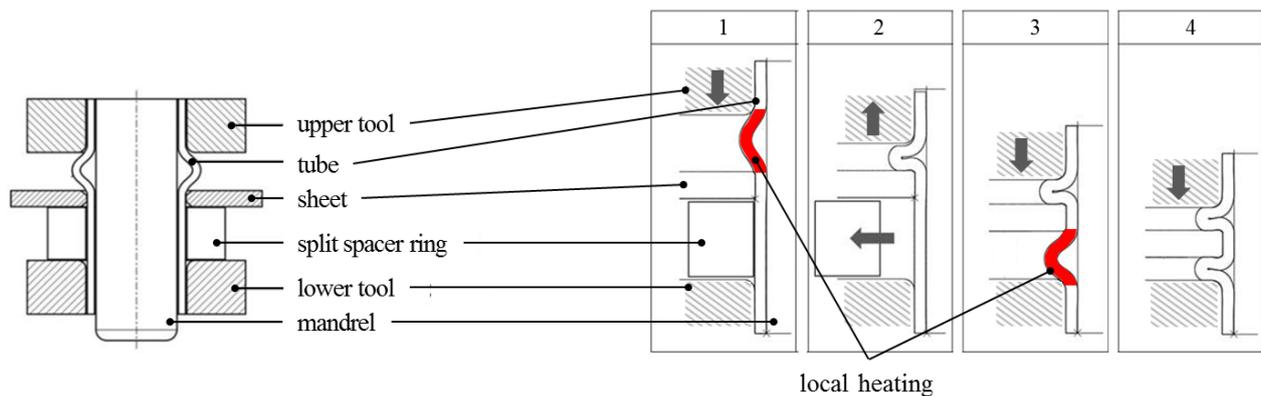
Fig. 8. Joining by upset bulging process aligned to local heating
