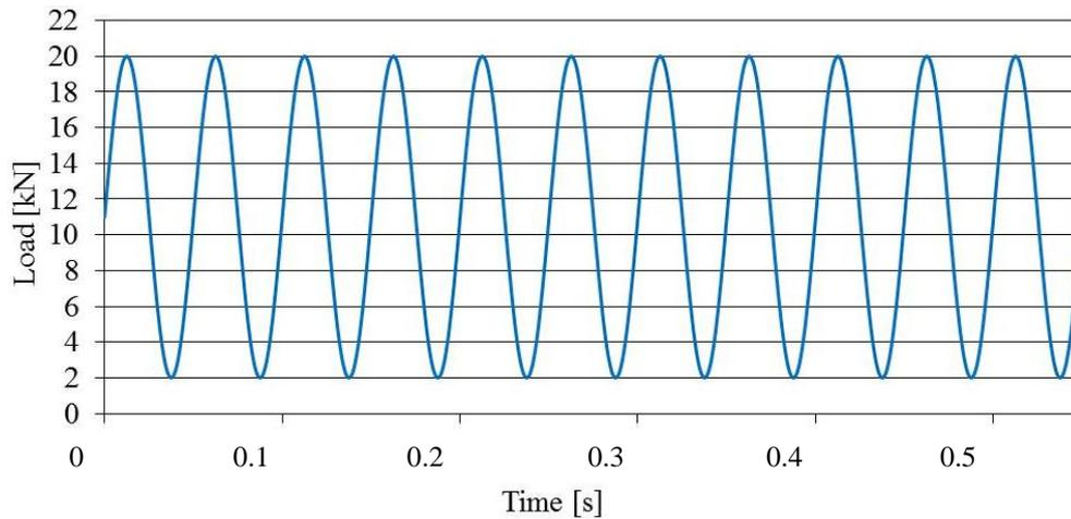
Fig. 11. Sinusoidal function of force during dynamic testing
