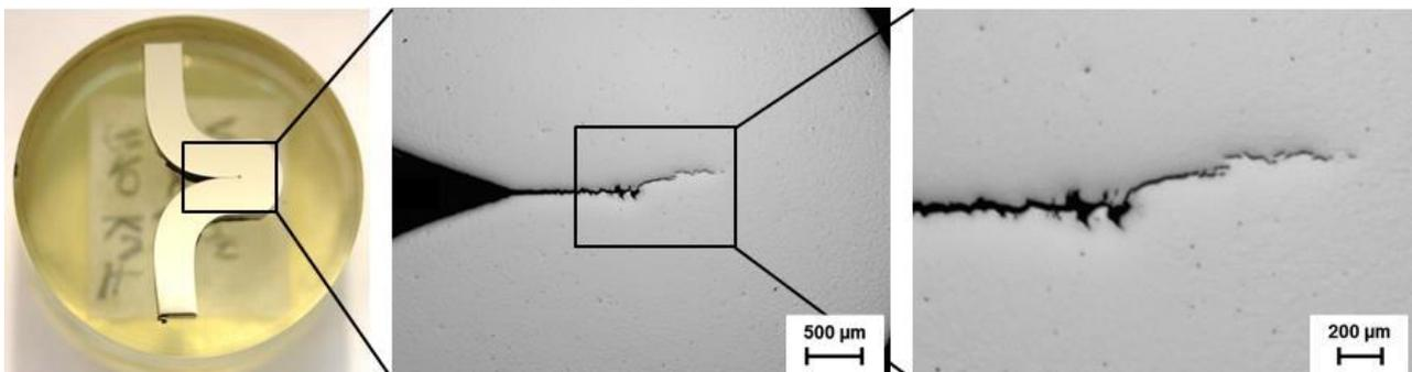
Fig. 5. Crack in the inner radius of a bulge formed at room temperature
