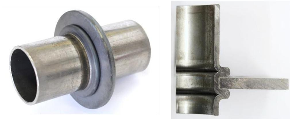
Fig. 9. Tube-to-sheet-joint – tube  $\text{\O}40 \times 2$  mm – sheet 5 mm
