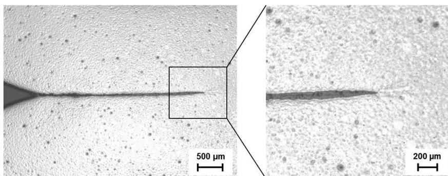
Fig. 10. Crack-free bulge formed at  $700^\circ\text{C}$
