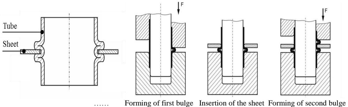
Fig. 1. Cross section of tube-sheet-joint and standard upset bulging process (schematic)
