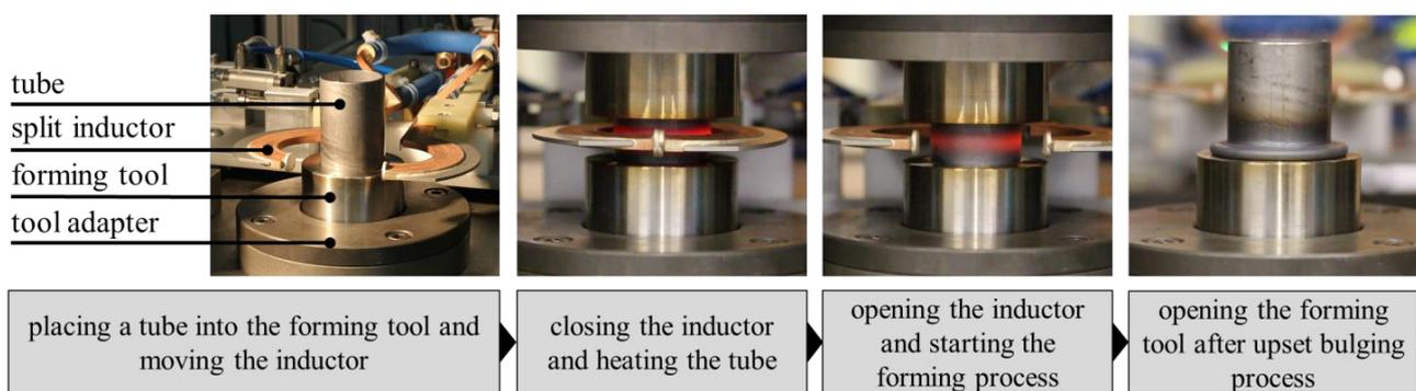
Fig. 6. Steps of the upset bulging process with local heating by split inductor
