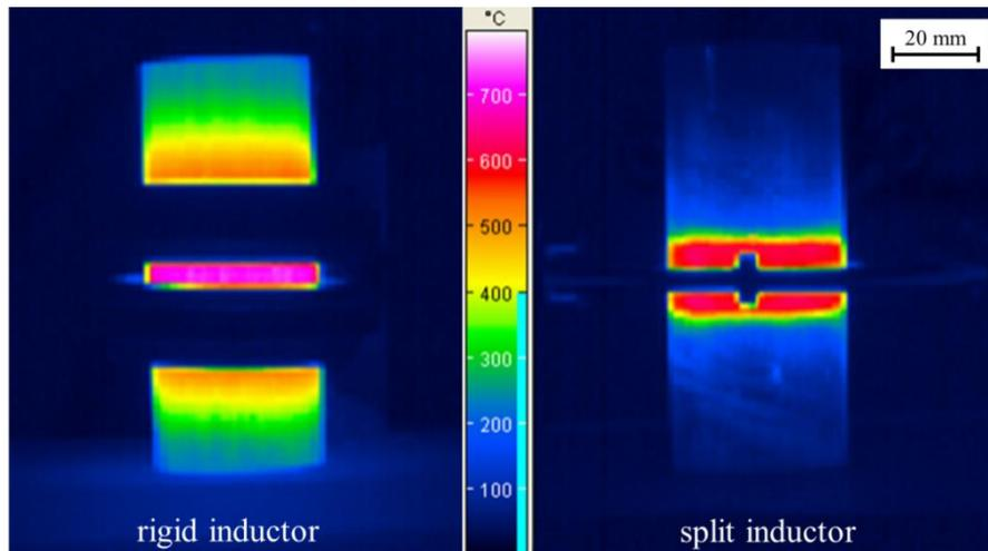
Fig. 7. Thermal images of the induction coils
