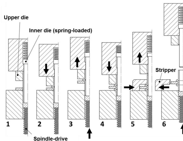
Fig. 3. Upset bulging prototyping tool for manufacturing tests
