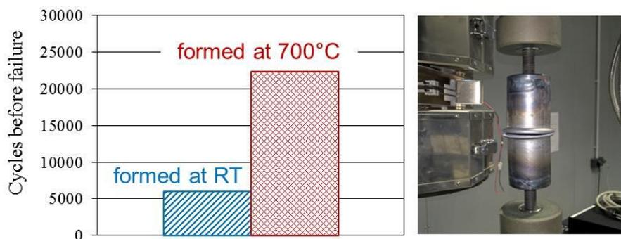
Fig. 12. Left: Cycles before failure for dynamic testing, Right: Sample at the end of testing
