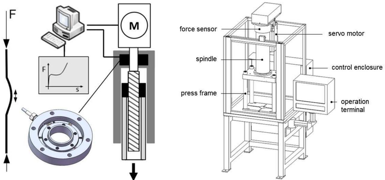
Fig. 2. Structure of a servo spindle press
