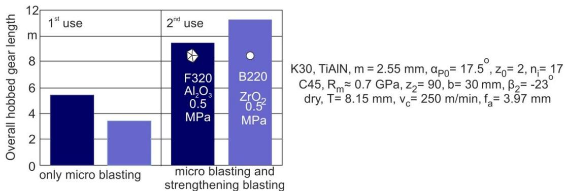
Fig. 6. Cutting performance of coated micro-blasted HM hobs, with various grain sizes and shapes
