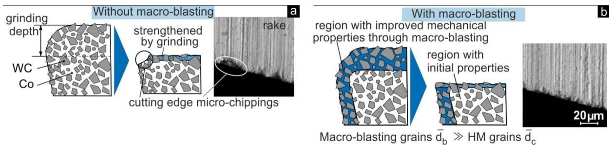
Fig. 5. Effect of macro-blasting and regrinding of the hob tooth rakes on the cutting edge sharpness
