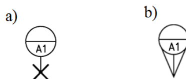
Fig. 2. a) fixed datum target, b) moveable datum target [1]
