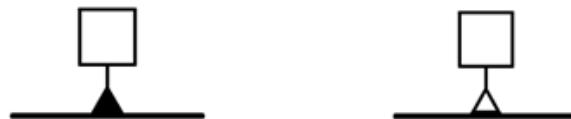
Fig. 1. Datum feature indicator: a box linked to a filled or open datum triangle by a leader line [1]
