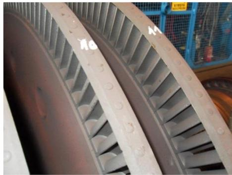
Fig. 1. Rotor disc of the 11<sup>th</sup> turbine stage
