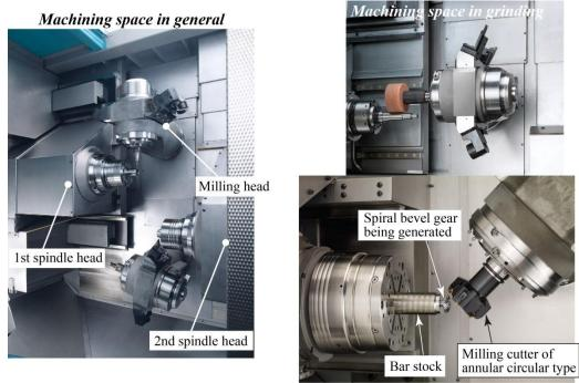
Machining space in spiral bevel gear cutting
