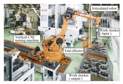
Fig. 8. Robot allocated at front of machine tool (by courtesy of Fujikoshi, 2010)
