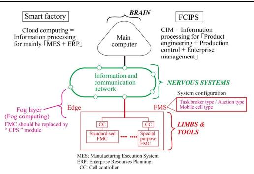
Fig. 1. Concept comparison of FCIPS with smart factory and their human-mimetic models
