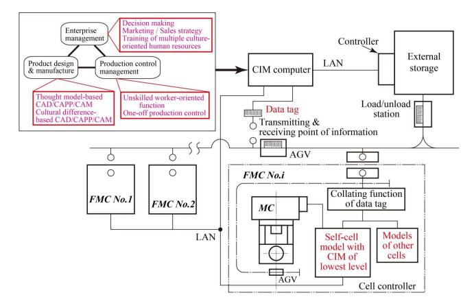
Fig. 2. Cell controller and information processing in FCIPS
