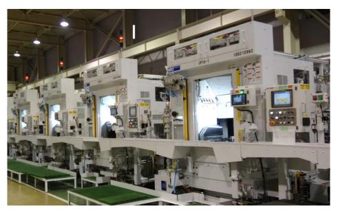
Fig. 12. FTL for cylinder block machining (by courtesy of Komatsu NTC, 2017)
