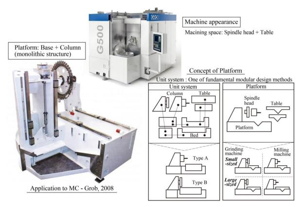
Fig. 15. Concept of "Platform" and its application to MC
