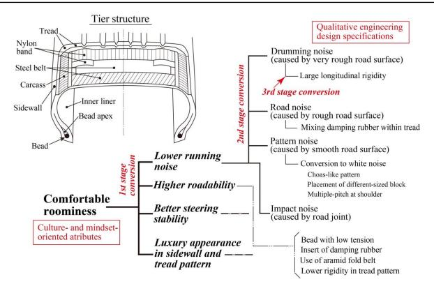
Fig. 17. Hierarchical tree structure representing conversion procedure of culture- and mindset-oriented attributes to engineering design requirements – in case of tier
