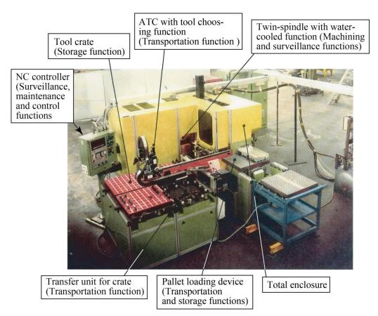
Fig. 14. System-function integrated MC of twin-spindle type (Type AUTOMAX I, by courtesy of MPM)
