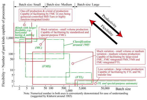
Fig. 7. Classification of flexible machining systems in 2010s
