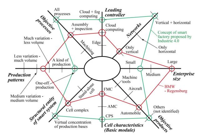
Fig. 3. Comparison of practical application by BMW with original concept proposed by "acatech"
