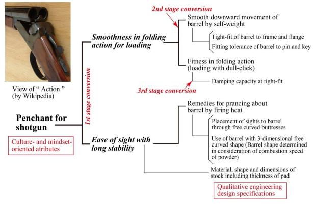
Fig. 18. Hierarchical tree structure representing conversion procedure of culture- and mindset-oriented attributes to engineering design requirements – in case of shotgun
