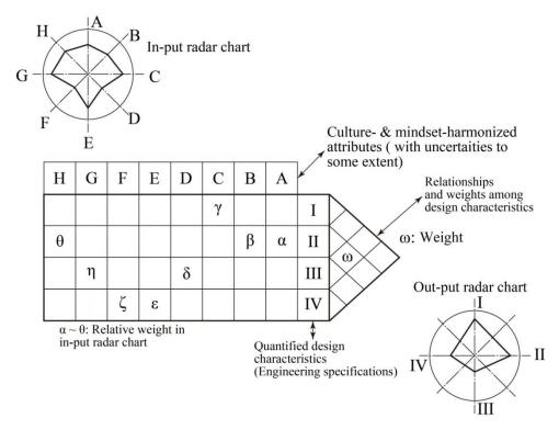
Fig. 20. Conversion method from culture- and mindset-harmonized attributes to engineering specifications by QFD of hierarchical type and radar chart (by Höft)
