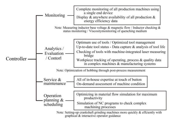
Fig. 4. Controller compatible with Industrie 4.0 - EMAG-brand, 2016
