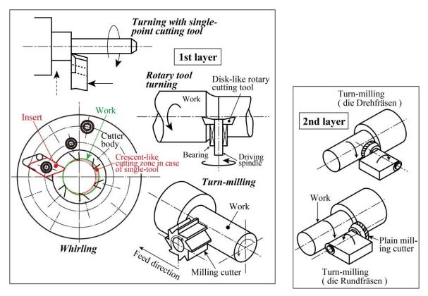
Fig. 19. Various turning methods to generate cylindrical component
