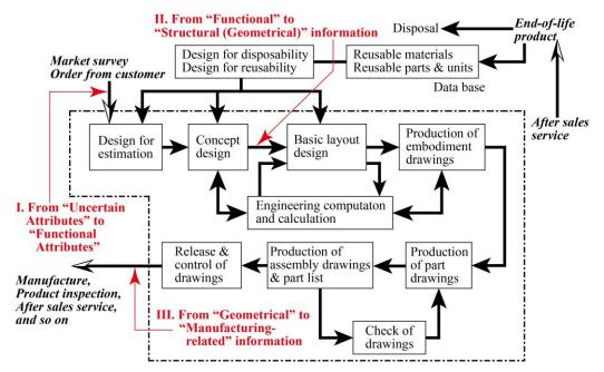
Fig. 16. Simplified flow in engineering design for product and several processes with property change in information
