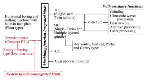
Fig. 10. A classification of "Highly Function-integrated Kinds" in 2010s
