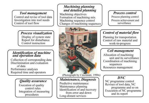
Fig. 5. Functionalities of FMS controller in general (by Uhlmann, 2008)
