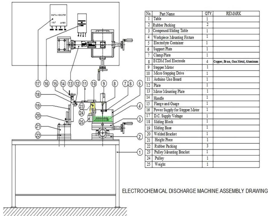
Fig. 11. ECDM Machine Assembly
