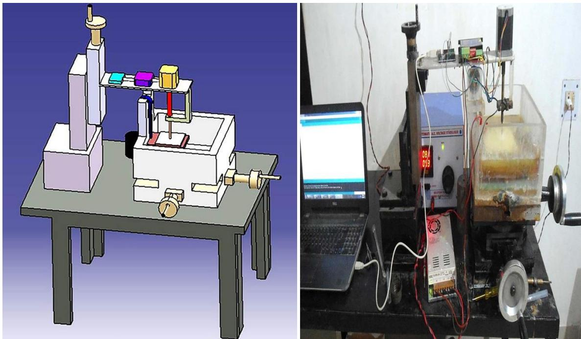
Fig. 13. ECDM Model and Manufactured ECDM machine setup
