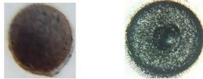
**Microscopic images of micro holes on ceramic and glass material using ECDM**
