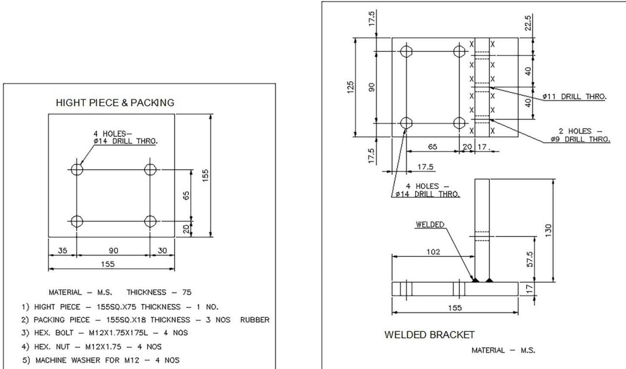
Fig. 6. Height piece and Welded bracket
