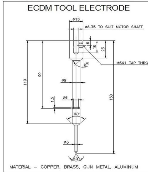
Fig. 10. ECDM Cathode Tool Electrode
