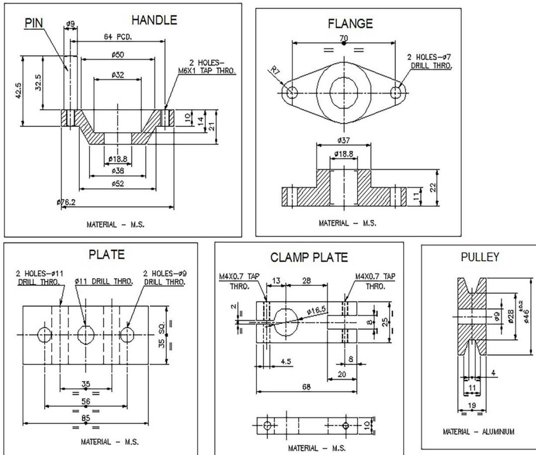
Fig. 9. Handle, Plate, Flange, Clamping plate and Pulley
