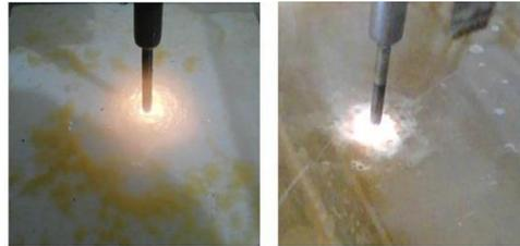
**Sparking during micro drilling on ceramic and glass material**
