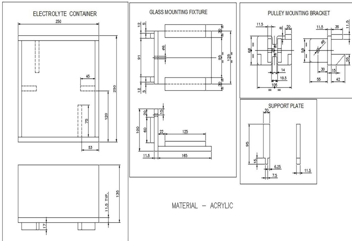
Fig. 5. Electrolyte container, Workpiece mounting fixture, Pulley mounting bracket and Support plate
