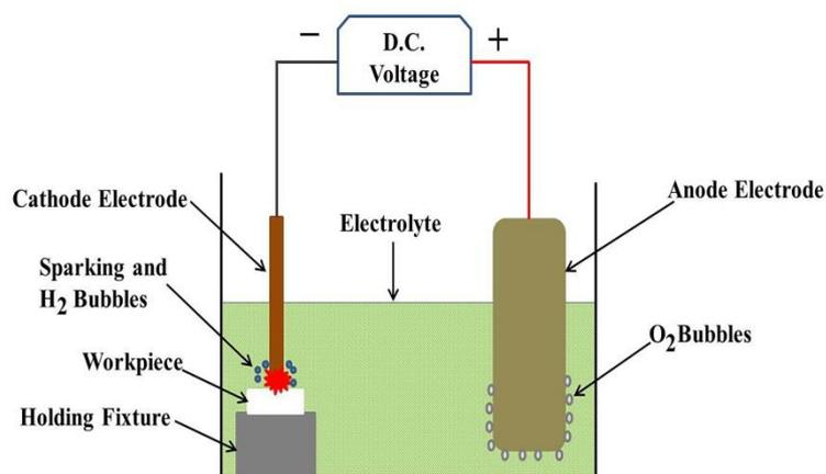
Fig. 1. Basic mechanism of ECDM process
