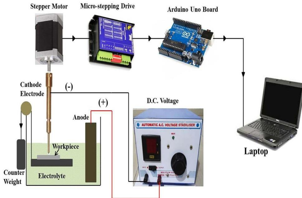
Fig. 2. Schematic diagram of ECDM machine setup
