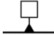
Fig. 1. Datum 1 cm. A box linked to a filled triangle by a leader line [14]
