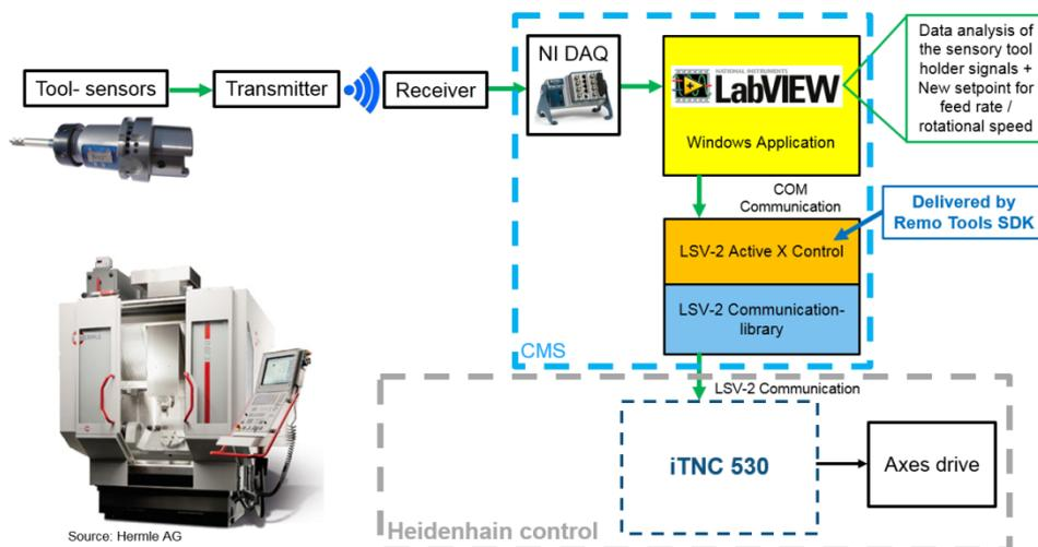
Fig. 7. Interfaces and data flow for a Heidenhain control system
