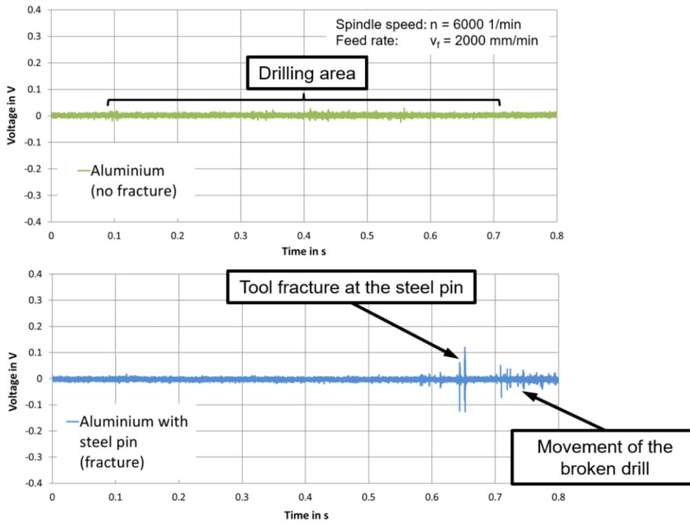
Fig. 5. Drilling in Aluminium (AlMg 3) with an interfering contour to initiate a tool fracture
