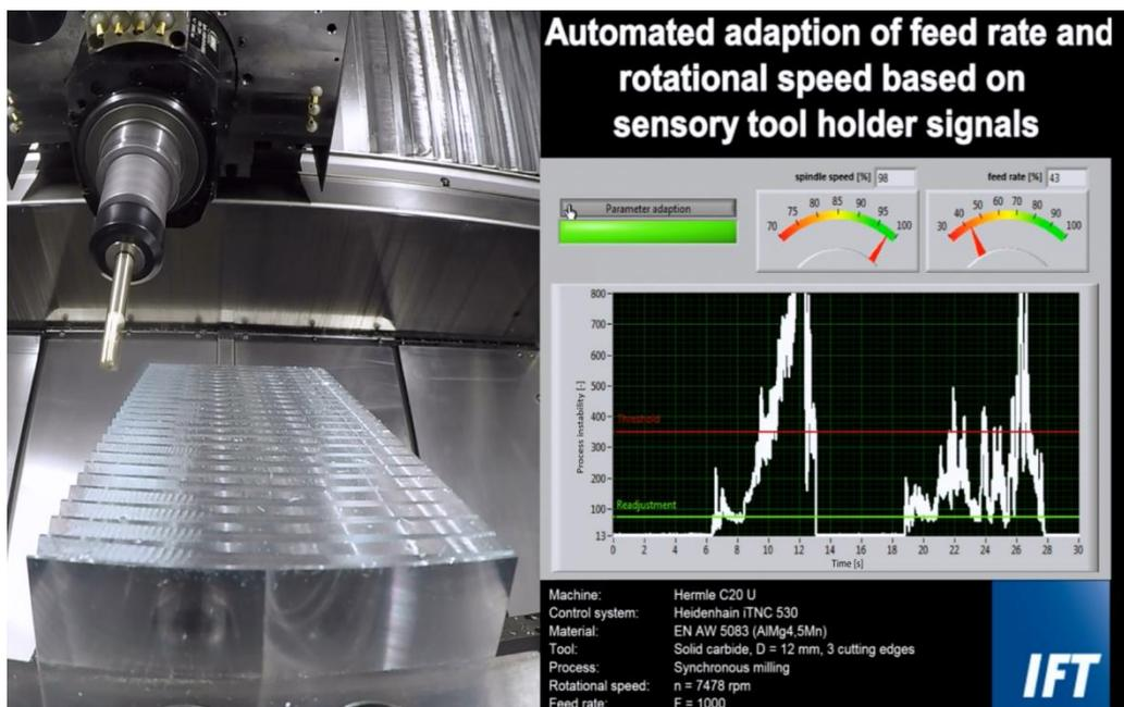
Fig. 8. Stability lobe experiment with automated adaption of parameters
