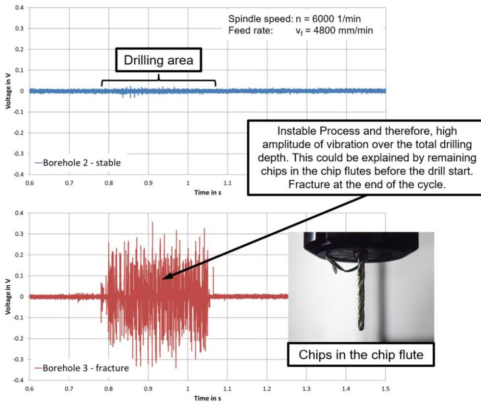
Fig. 6. Drilling in Aluminium (AlMg 3) until the occurrence of a tool fracture
