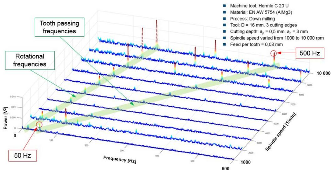
Fig. 4. Signals of the balanced sensory tool holder up to 10.000 rpm
