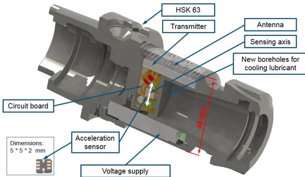
Fig. 3. Sectional view of the sensory tool holder
