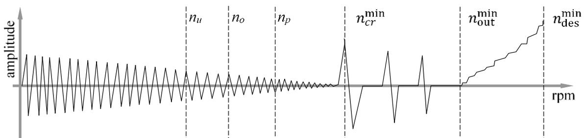
Fig. 1. Characteristic rotational speeds of the circular saw blade according to Stakhiev [17]:  $n_u$  – universal;  $n_o$  – optimal;  $n_p$  – permissible;  $n_{cr}^{\min}$  – the lowest critical;  $n_{out}^{\min}$  – the lowest self-excited;  $n_{des}^{\min}$  – destructive
