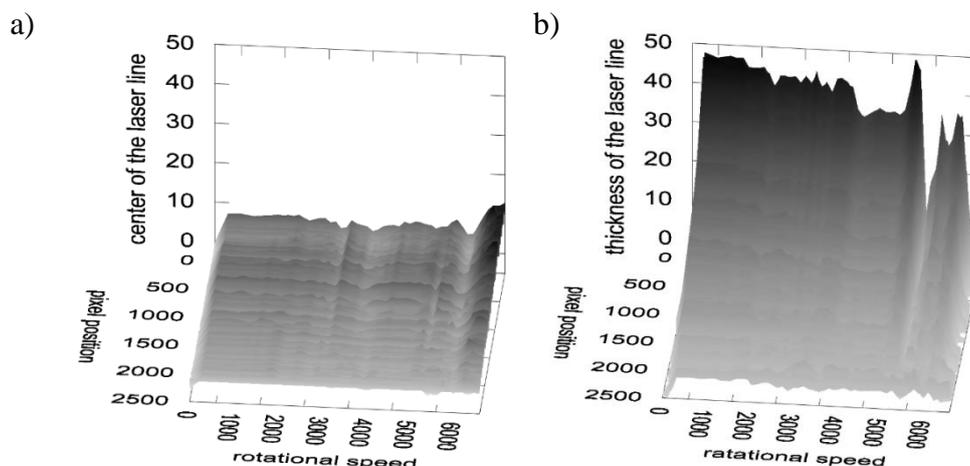
Fig. 6. Variations of the centre laser line in pixels (a) and laser line thickness in pixels (b) in a function of the spindle rotational speed
