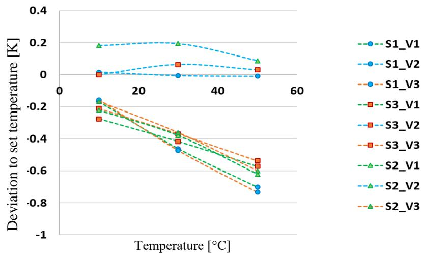
Fig. 6. Influence of electrical amplifier on sensor
