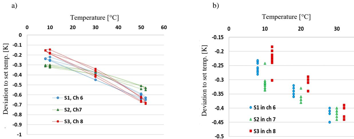
Fig. 3. a) Sensor response to rising and falling temperatures; b) Influence of sensors being re-plugged in channel repeatedly
