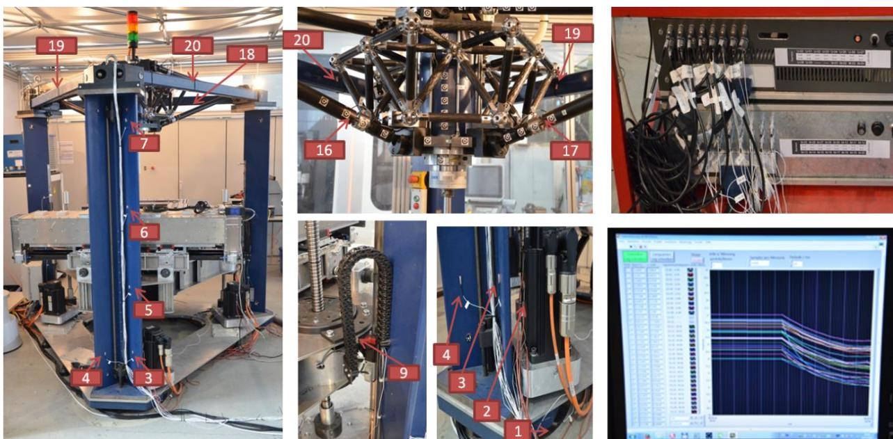
Fig.1. Application of PRT-sensors along a machine structure. On the right: multi-channel-readout and diagram of detected temperature
