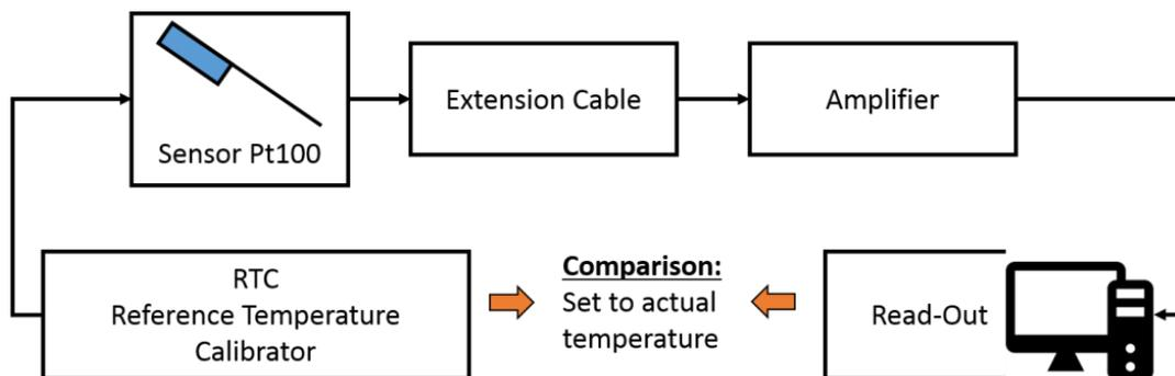
Fig. 2. Elements of measurement chain
