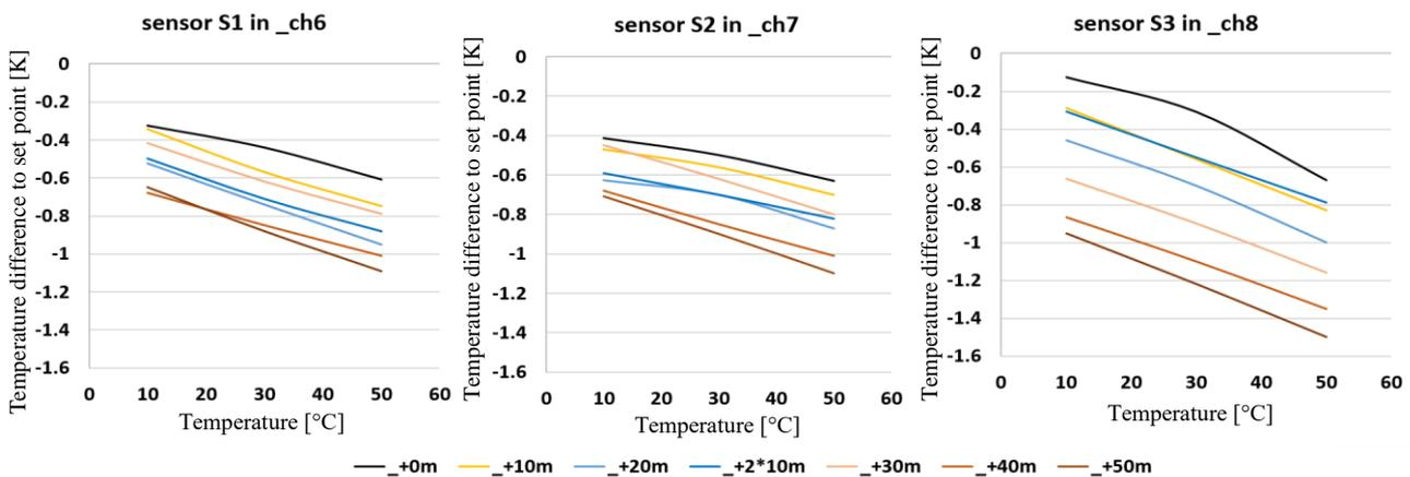
Fig. 5. Influence of different cable length on sensors
