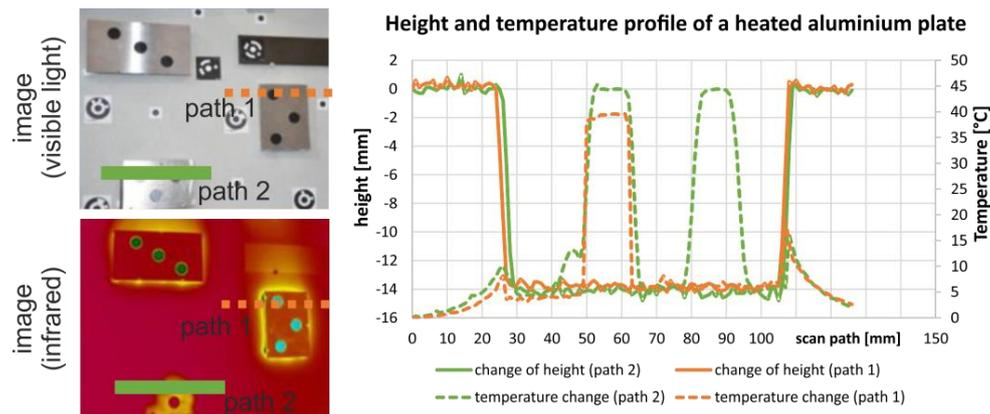
Fig. 9. Distance and temperature by two scans of two paths
