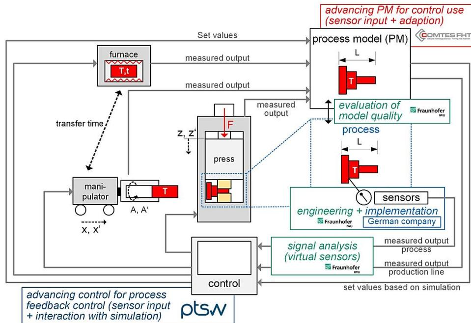
Fig. 3. Signal flow between the components
