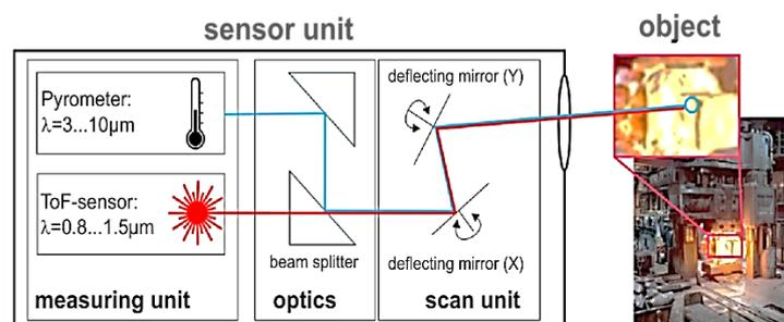
Fig. 7. Scanning device
