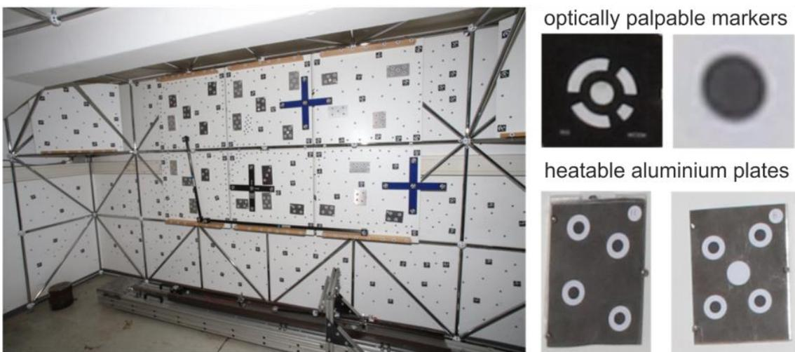
Fig. 8. Calibration wall with markers and heatable segments
