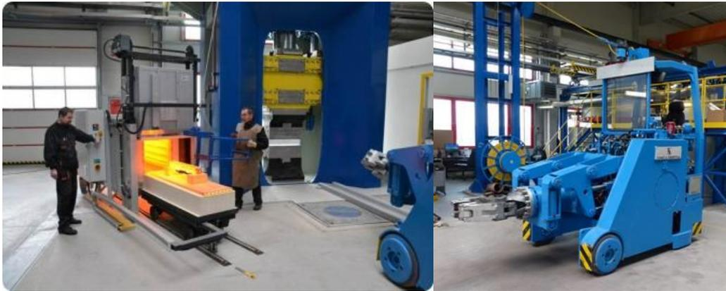
Fig. 2. Furnace, forging-press and manipulator in the project partner COMTES' facility [15]
