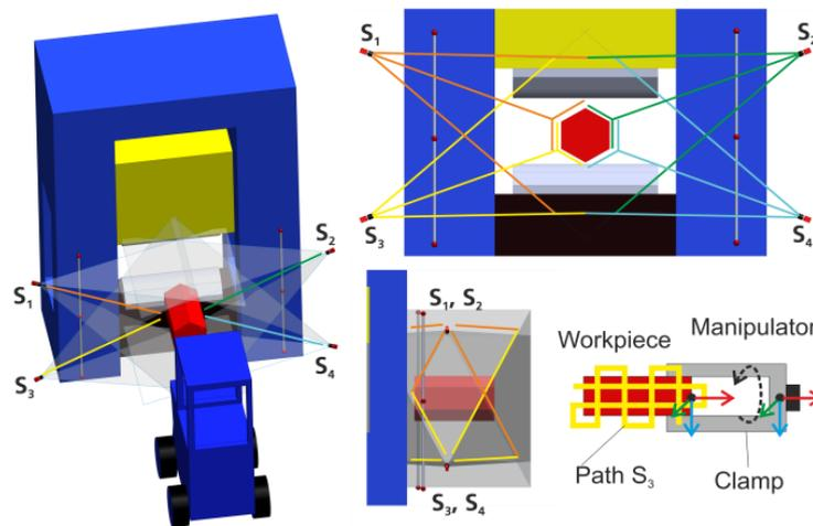
Fig. 6. Geometric restrictions at COMTES facility and scan path at the work piece
