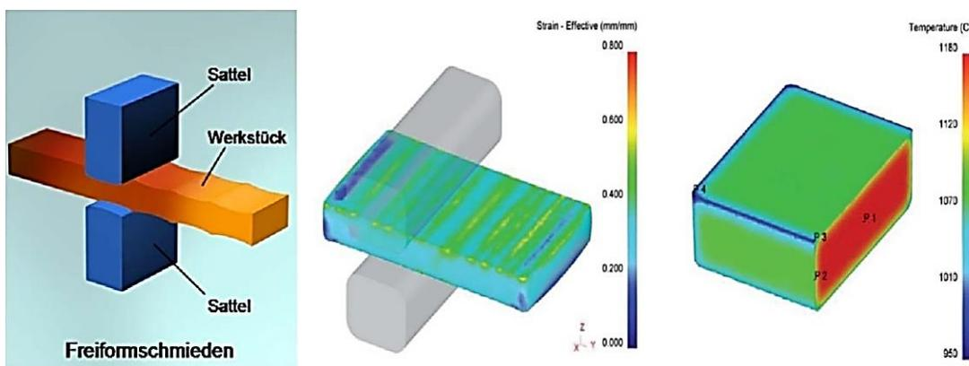
Fig. 1. Schematic representation of open-die forging (left, [1]), representation of the simulated component condition during the first forging phase (centre, [10]) and temperature distribution before the forging process (right, [10])
